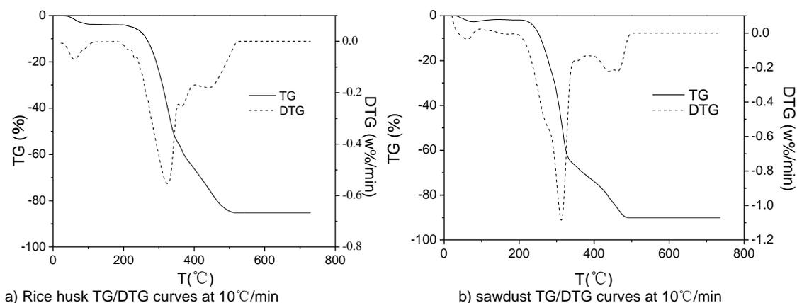
**Fig. 2.** Thermogravimetric analysis of rice husk and sawdust
