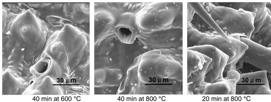
Fig. 8. SEM images of rice husk char at different char-making conditions (1,000x magnification)
