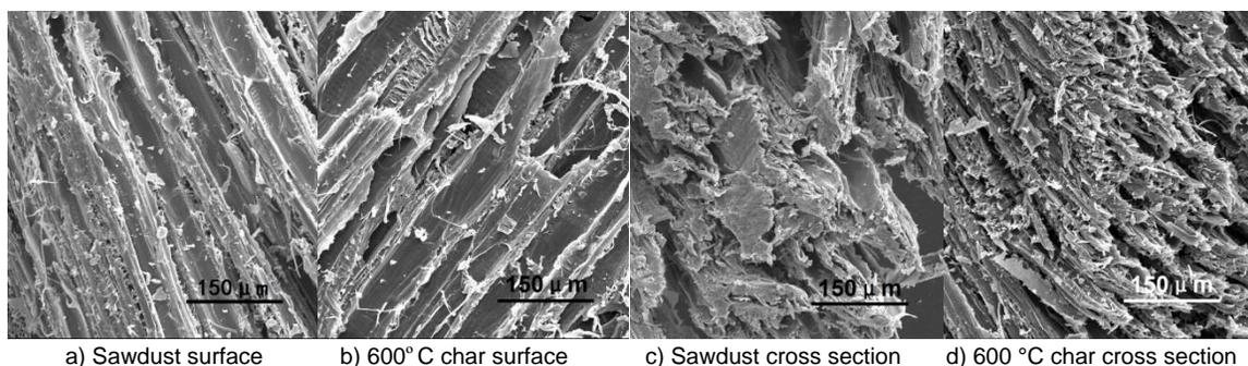
**Fig. 7.** SEM images of sawdust and its char (200× magnification)
