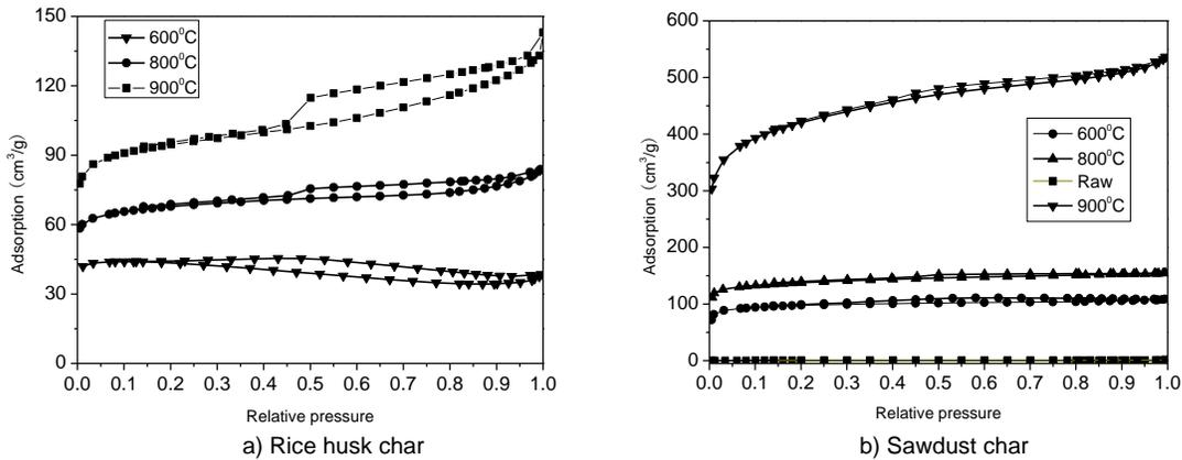
**Fig. 10.** Isothermal adsorption/desorption curves for rice husk char and sawdust char
