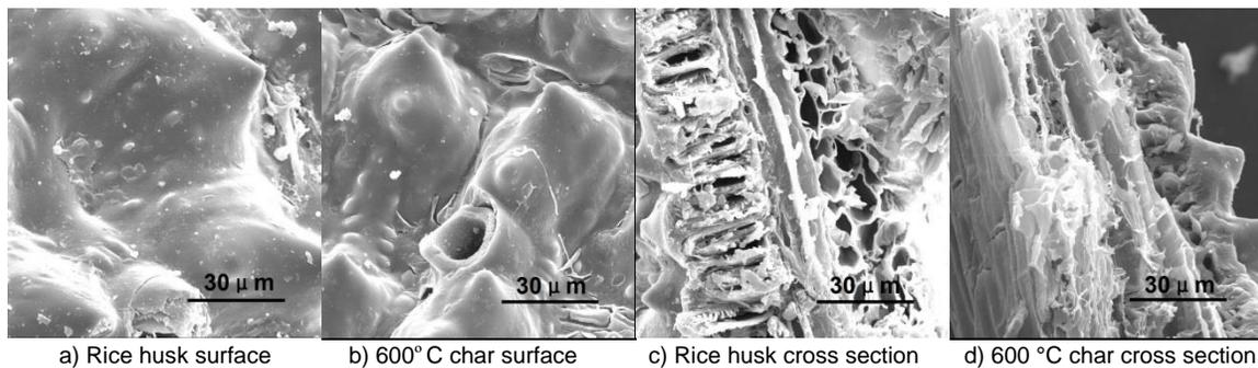
**Fig. 6.** SEM images of rice husk and its char (1,000× magnification)
