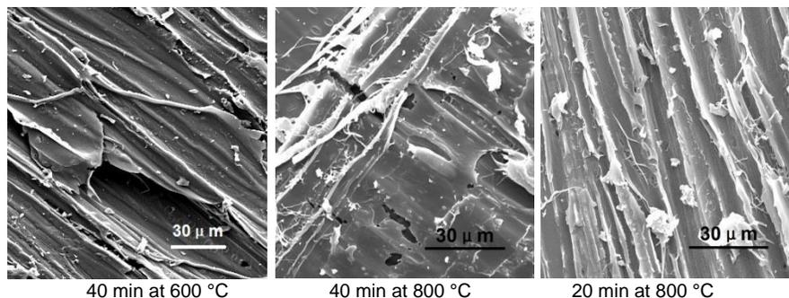
Fig. 9. SEM images of sawdust char at different char-making conditions (1,000x magnification)
