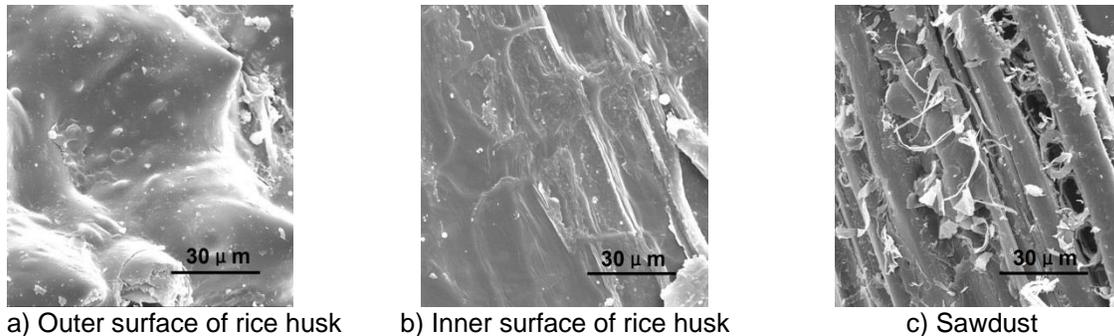
**Fig. 5.** SEM images of rice husk and sawdust (1000× magnification)
