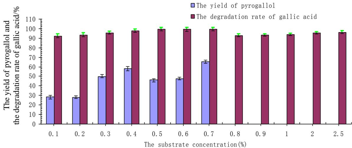
**Fig. 4.** Effects of substrate concentration on pyrogallol production (5% inoculum size, 25% phosphate buffer at 30 °C, cultivation for 60 h at pH 6.2, and 180 r/min shaking)
