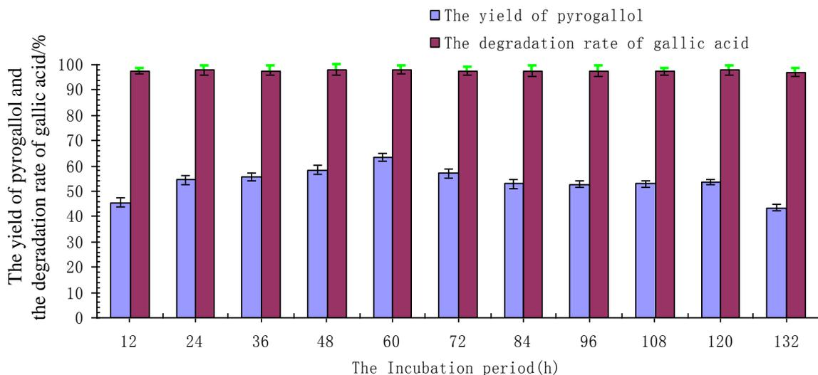
**Fig. 5.** Effects of incubation period on pyrogallol production (5% inoculum size, 0.4% gallic acid, 25% phosphate buffer, temperature of 30 °C, 6.2 pH value, and 180 r/min for shaking)
