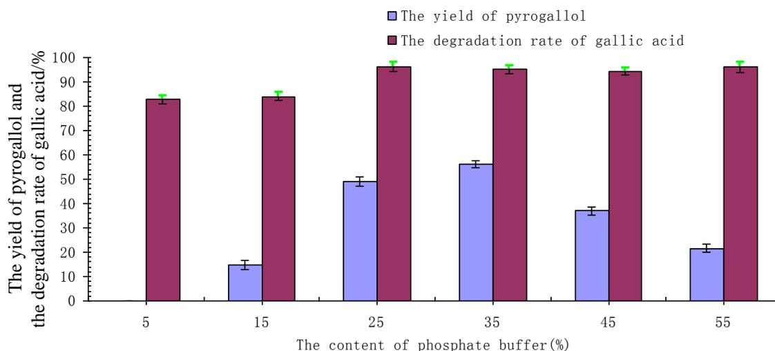
**Fig. 7.** Effect of phosphate buffer content on pyrogallol production (5% inoculum size, 0.4% gallic acid at 30°C, cultivated for 60 h at pH 6.2, and 180 r/min shaking)
