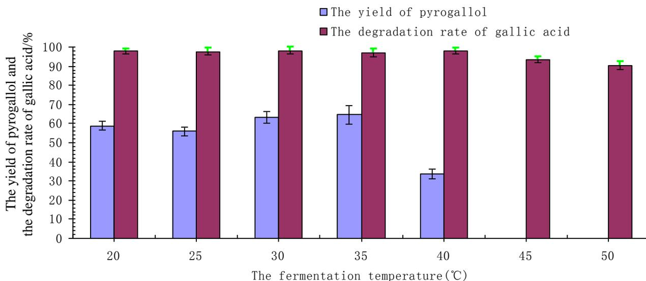
**Fig. 6.** Effect of fermentation temperature on pyrogallol production (5% inoculum size, 0.4% gallic acid, 25% phosphate buffer, cultivated for 60 h at pH 6.2, 180 r/min shaking)
