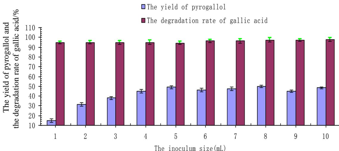
**Fig. 3.** Effect of inoculum size on pyrogallol production (0.2% gallic acid, 25% phosphate buffer, at 30°C, cultivated for 60 h at pH 6.2, and 180 r/min shaking)
