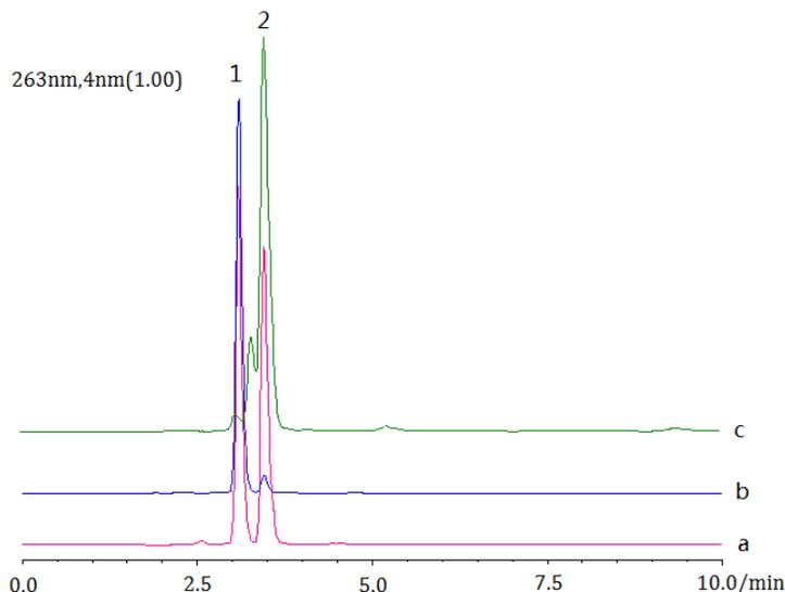
**Fig. 2.** Detection of pyrogallol from fermentation liquor by HPLC: (a) mixed standards of gallic acid and pyrogallol; (b) after 48 h of fermentation; (c) after 60 h of fermentation
