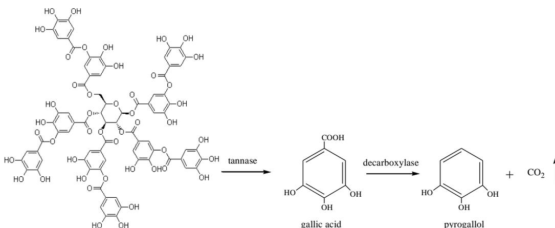
**Fig. 1.** The route of degradation of gallic acid to produce pyrogallol
