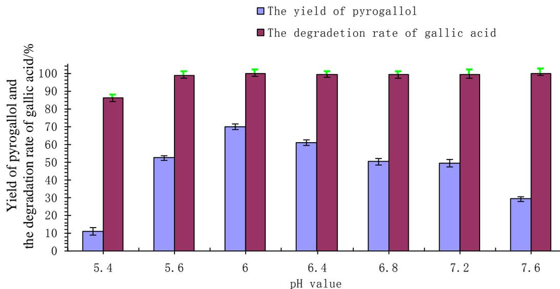
**Fig. 8.** Effect of pH value on pyrogallol production (5% inoculum size, 0.4% gallic acid at 30°C, cultivated for 60 h with 25% phosphate buffer, and 180 r/min shaking)
