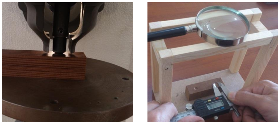
Fig. 2. Brinell hardness test and measurement of the indentation diameter
