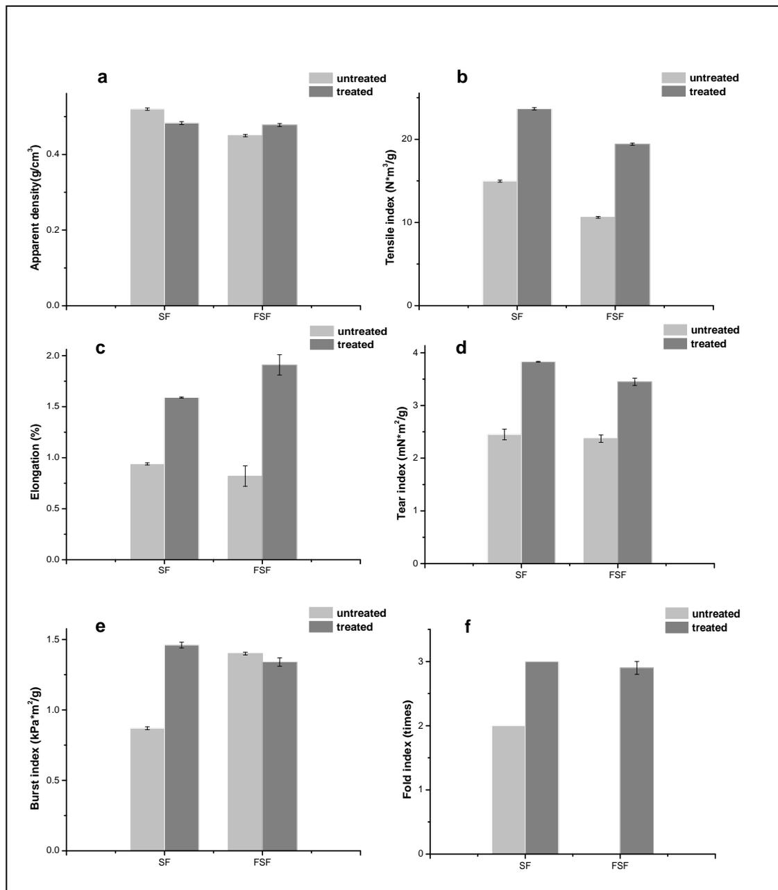
**Fig. 2.** Comparison of sheet physical properties: (a) tightness, (b) tensile index, (c) elongation, (d) tear index, (e) burst index, and (f) fold index
