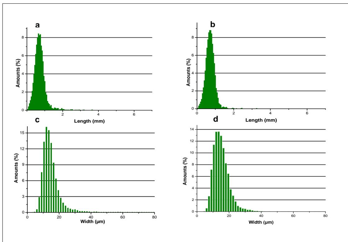
**Fig. 1.** The length and width distribution of SF and FSF. (a) the length distribution of SF, (b) the length distribution of FSF, (c) the width distribution of SF, and (d) the width distribution of FSF
