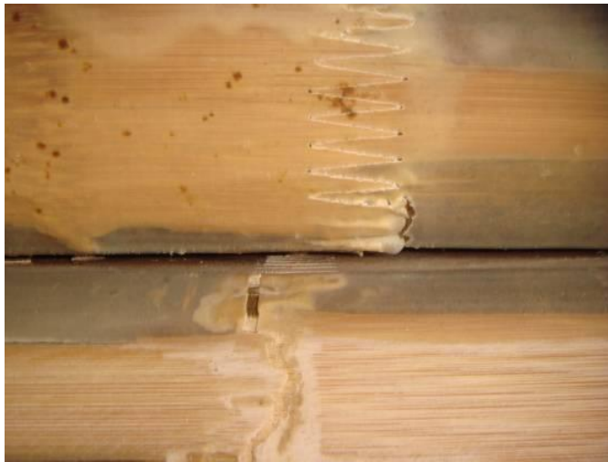
Fig. 6. Transverse bending loading failure of GPEHB
