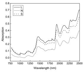
Fig. 1. The mean spectra from original data of large knots (L), small knots (S), and knot-free samples (N)
