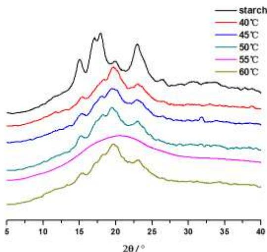
**Fig. 3.** X-ray diffraction patterns of the corn starch and treated starch samples
