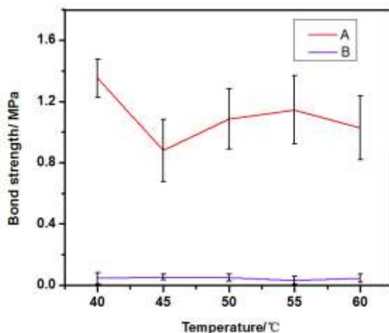
**Fig. 1.** Effects of treatment temperature on bond strength of starch adhesives A: starch treated with pMDI B: starch treated without pMDI
