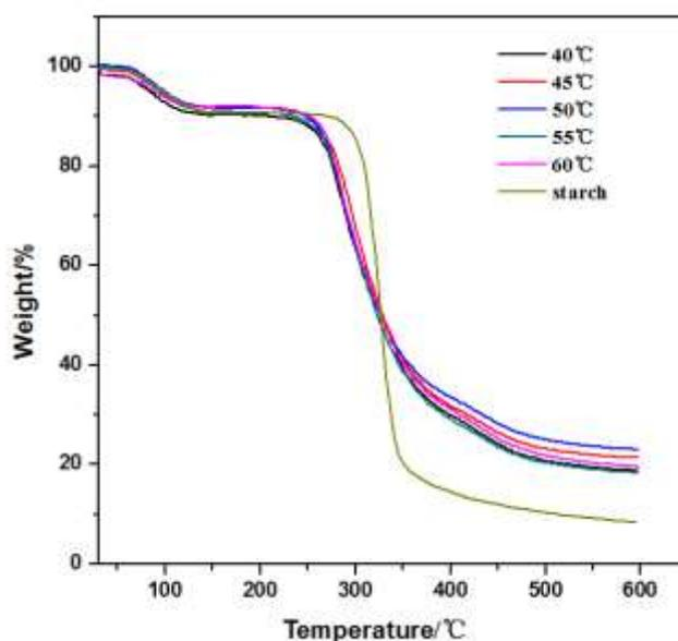
**Fig. 5.** TGA curves of starch and treated starch samples
