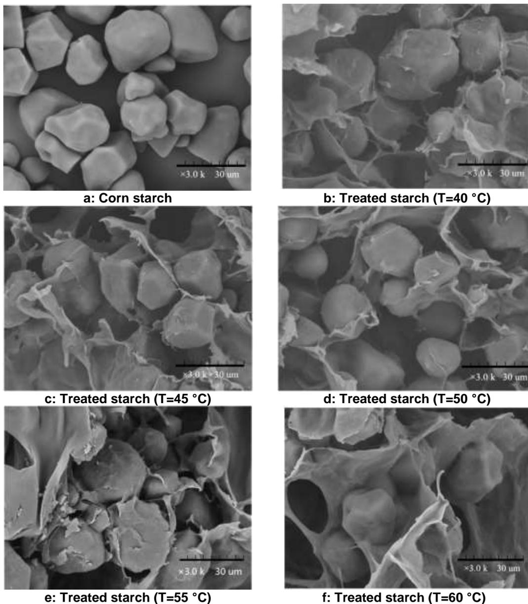
**Fig. 4.** Scanning electron micrographs of corn starch and treated starch samples
