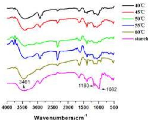
**Fig. 2.** FTIR spectra of corn starch and treated starch
