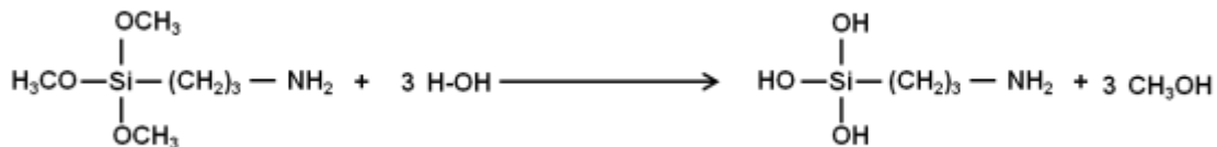
a) Hydrolysis of silane to silanol
