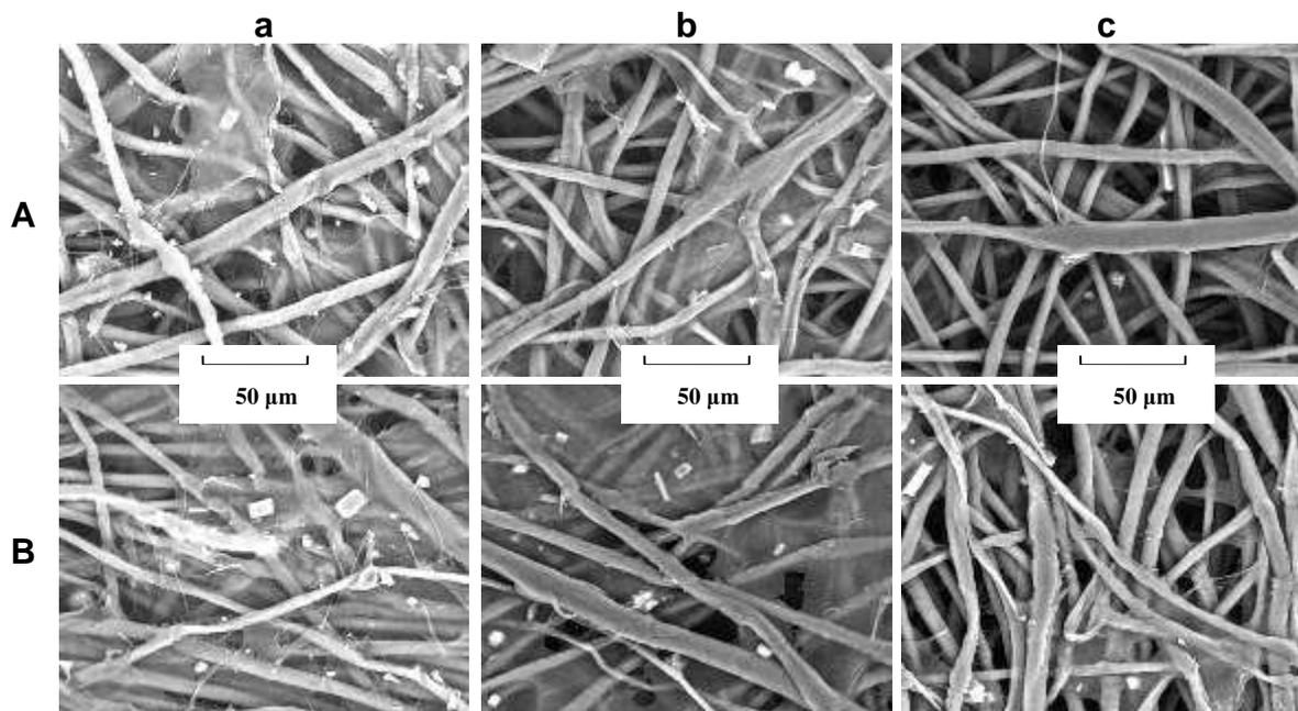
**Fig. 3.** SEM micrographs obtained for (A) gampi soda pulp and (B) gampi soda pulp with oxalate for (a) unbleached pulps, (b) 0.15 Kappa factor  $\text{ClO}_2$  bleached pulps, and (c) after 0.15 Kappa factor  $\text{ClO}_2$  bleaching with pectinase BL11 260 IU/g.o.d.p. pretreatment
