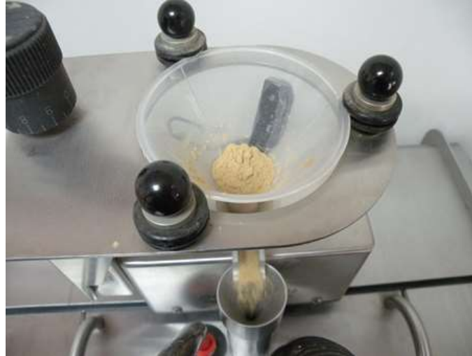
Fig. 2. Sample analysis using the Laser Particle Sizer Analysette 22 MicroTec plus
