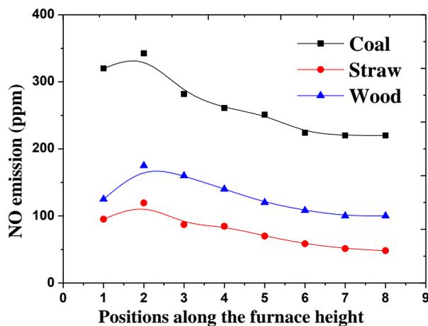
Fig. 3. Axial NO concentration profiles of coal/straw/wood combustion
