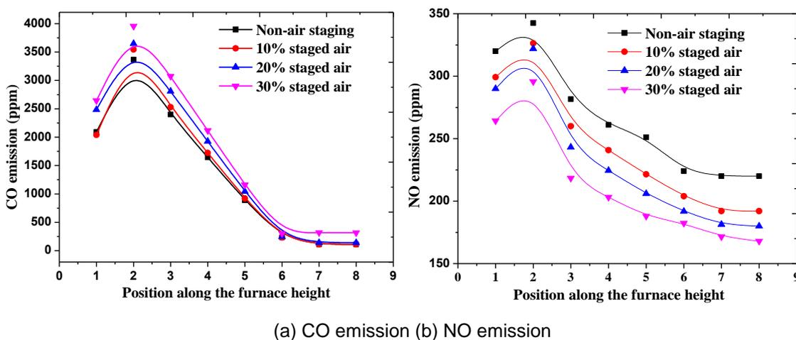
**Fig. 6.** Effect of air staging ratio on CO and NO emission in coal combustion
