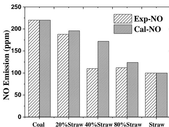
**Fig. 4.** Effect of biomass co-firing ratio on NO emission
