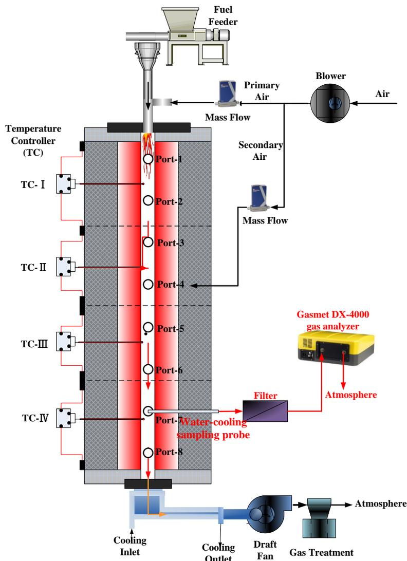
**Fig. 1.** Experimental system of drop tube furnace
