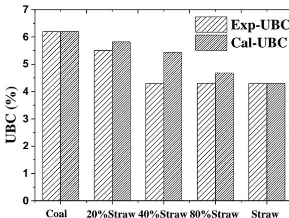
**Fig. 5.** Effect of biomass co-firing ratio on UBC
