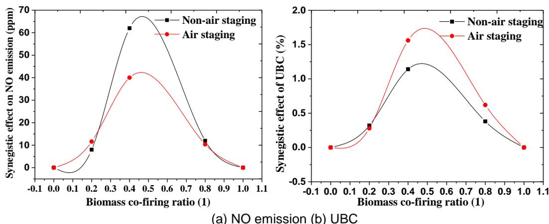
Fig. 9. Effect of biomass co-firing ratio on the synergetic effect
