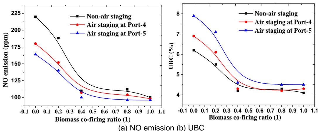
Fig. 8. Effect of co-firing ratio on NO emission and UBC with 20% air staging
