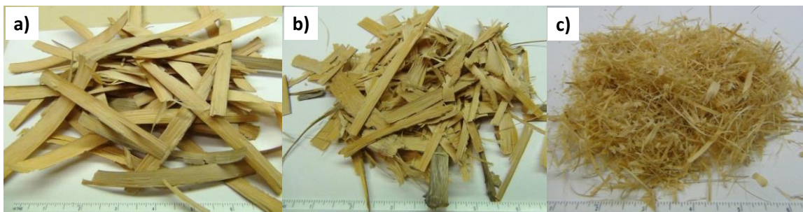
Fig. 6. Appearance of moso bamboo: (a) strands (>14.3-mm); (b) large fines (7.8-mm to 14.3-mm); and (c) small fines (3.18-mm to 7.8-mm)
