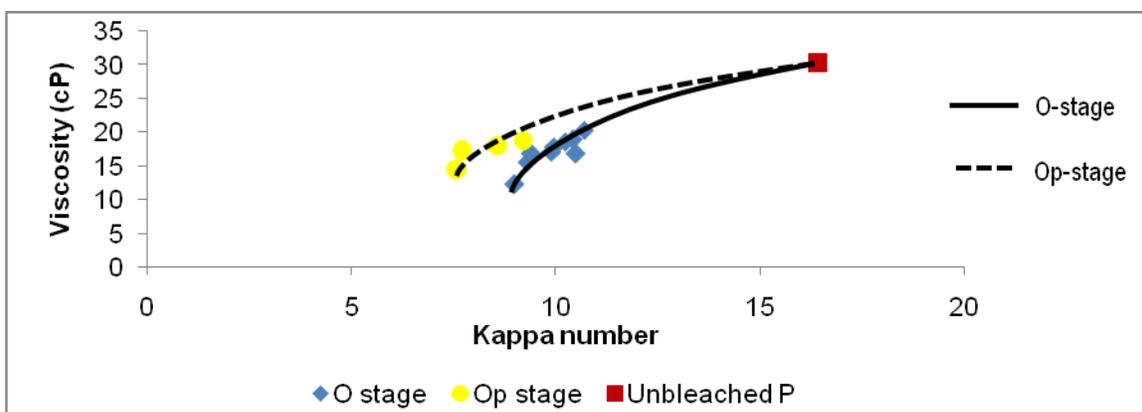
Fig. 1. Selectivity plot of O-stage and Op-stage on hardwood kraft pulp
