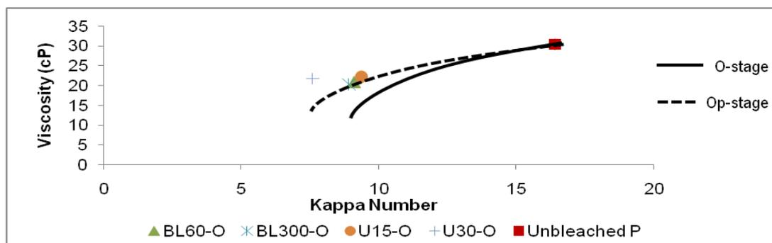
**Fig. 2.** Study of the selectivity plot of blue light and ultraviolet photo pre-treatment of the O-stage on hardwood kraft pulp
