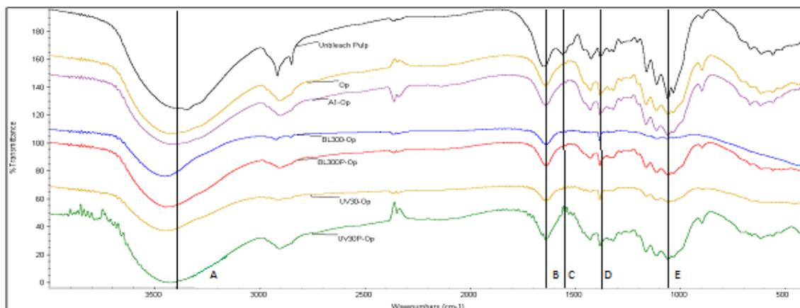
Fig. 8. Distribution area for the assignment band of the signal in FTIR spectra on photo pre-treated Op-stage pulp (A refers to hydroxyl groups ( $3400\text{ cm}^{-1}$ ); B refers to carbonyl groups ( $1650\text{ cm}^{-1}$ ); C refers to aromatic groups ( $1550\text{ cm}^{-1}$ ); D refers to S unit ( $1380\text{ cm}^{-1}$ ), and E refers to carbon-oxygen bond ( $1160\text{ cm}^{-1}$ ))
