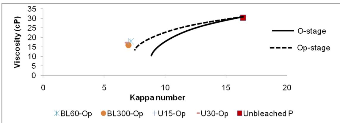
Fig. 6. Selectivity plot of blue light and ultraviolet photo pre-treatment with the Op-stage on hardwood kraft pulp
