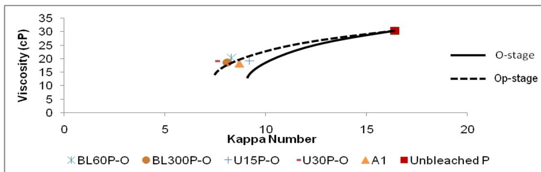
**Fig. 4.** Selectivity plot of PAA-aided blue light and ultraviolet photo pre-treatment with the O-stage on hardwood kraft pulp
