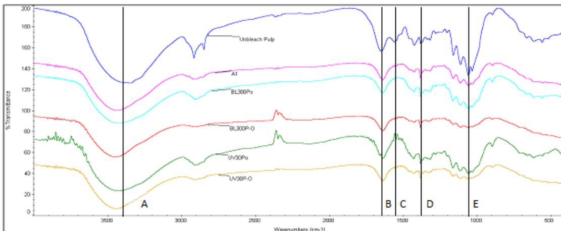
**Fig. 5.** Distribution area for the assignment band of the signal in FTIR spectra of PAA-aided photo pre-treated oxygen delignified pulp (A refers to hydroxyl groups ( $3400\text{ cm}^{-1}$ ); B refers to carbonyl groups ( $1650\text{ cm}^{-1}$ ); C refers to aromatic groups ( $1550\text{ cm}^{-1}$ ); D refers to S unit ( $1380\text{ cm}^{-1}$ ), and E refers to carbon-oxygen bond ( $1160\text{ cm}^{-1}$ ))
