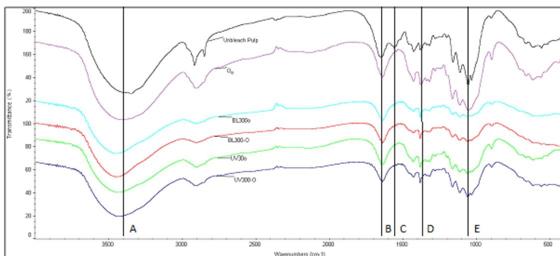
**Fig. 3.** Distribution area for the assignment band of the signal in the FTIR spectra of photo pre-treated oxygen-delignified pulp. (A refers to hydroxyl groups ( $3400\text{ cm}^{-1}$ ); B refers to carbonyl groups ( $1650\text{ cm}^{-1}$ ); C refers to aromatic groups ( $1550\text{ cm}^{-1}$ ); D refers to S unit ( $1380\text{ cm}^{-1}$ ), and E refers to carbon-oxygen bond ( $1160\text{ cm}^{-1}$ ))
