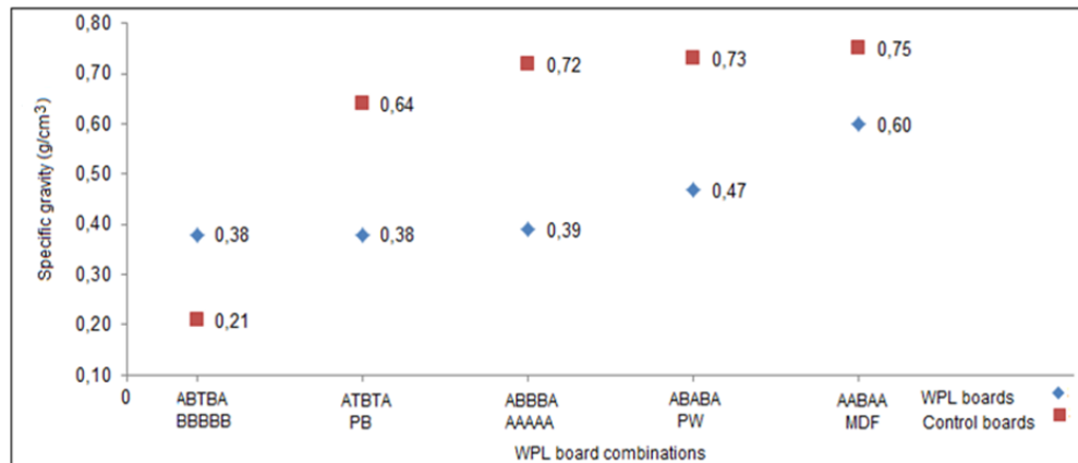
Fig. 5. Determination of the specific gravity
