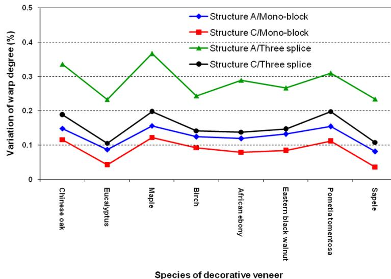
**Fig. 6.** The effect of surface wood species and type of core layer on warping deformation for engineered wood floorings
