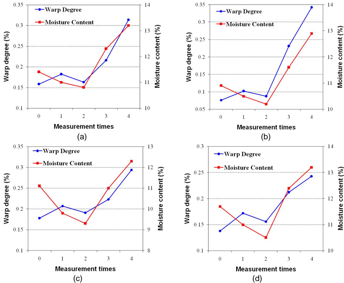
**Fig. 7.** The variation trend for the degree of warping and the moisture content (%): (a) structure A with mono-block and maple, (b) structure A with three splice and eastern black walnut, (c) structure C with mono-block and Chinese oak, and (d) structure C with three splice and eucalyptus
