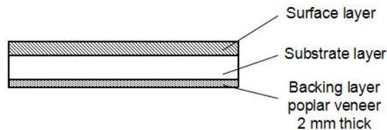
**Fig. 1.** Three layer construction of engineered wood flooring
