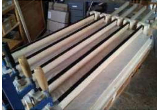
Fig. 1. Method of pre-stressing timber beams
