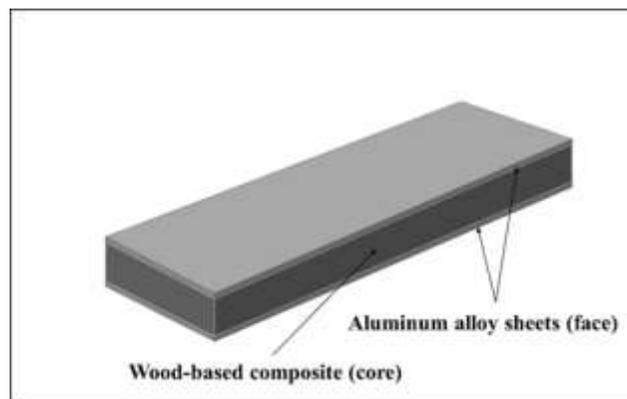
**Fig. 1.** Schematic illustration of aluminum-laminated panel
