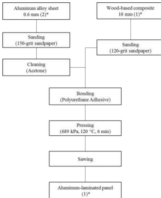
**Fig. 3.** Manufacturing process of aluminum-laminated panels. \*Quantity of material
