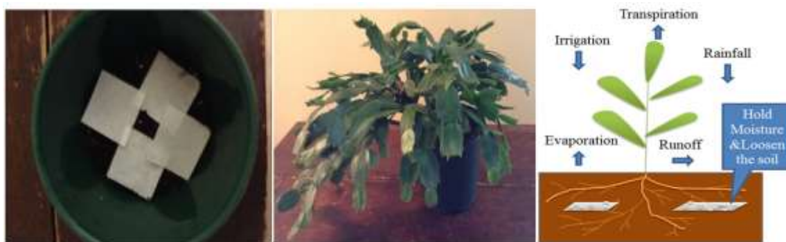
Fig. 6. Schematic for using the paper/PAA composites in plant pot/bedding (Left: the actual paper/PAA composites with 2 g/m 2 PAA hydrogel loading; Middle: plant in a pot with paper/PAA composites as bedding; Right: explanation of paper/PAA composites as plant bedding)
