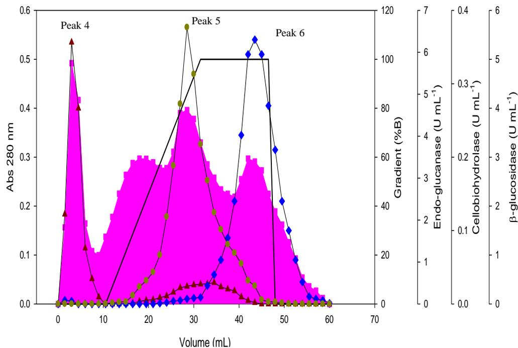
**Fig. 5.** Protein purification from the culture filtrate by hydrophobic chromatography using a HiTrap Phenyl FF column. Distribution of the protein and elution profile of the proteins recorded at 280 nm (■); profile of the 50 mM NaAc gradient (—) on endoglucanases (▲), cellobiohydrolase (◆), and β-glucosidase (●)
