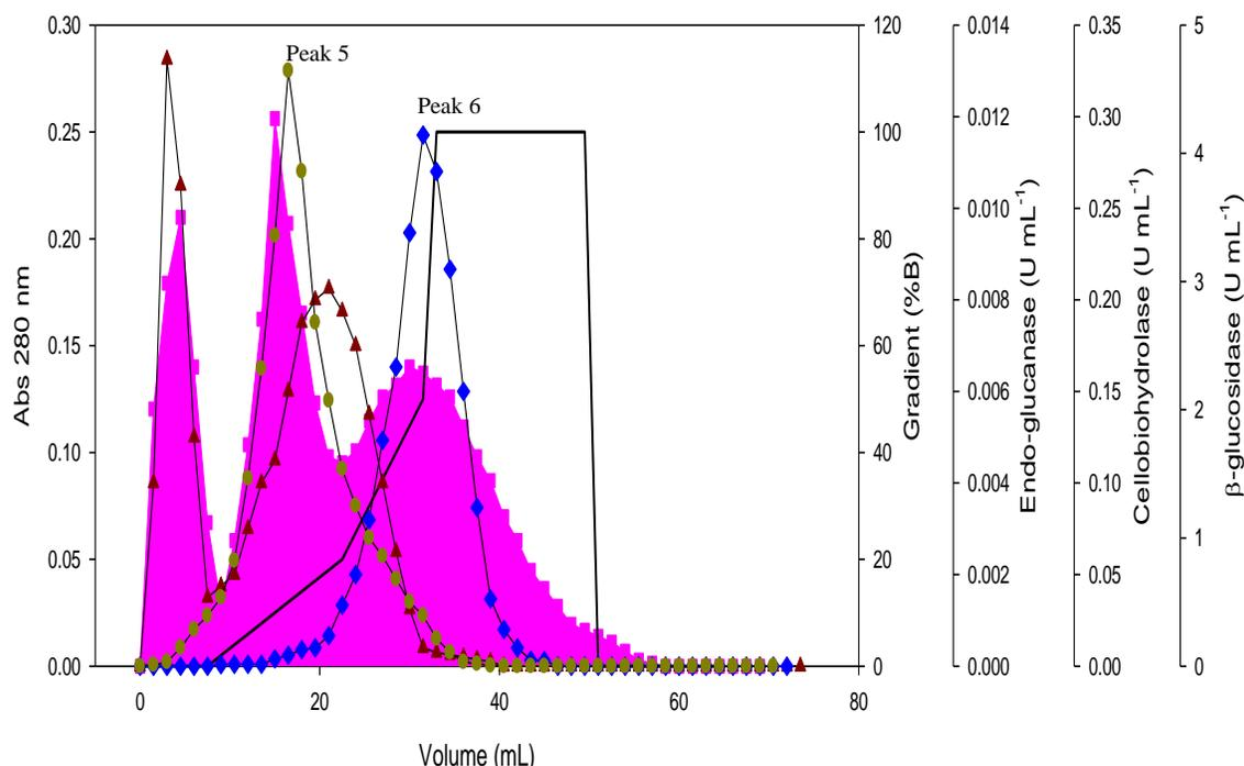
**Fig. 6.** Protein purification from the culture filtrate by cation exchange chromatography using a HiTrap SP FF column. Distribution of the protein and elution profile of the proteins recorded at 280 nm (■); profile of the 1 M NaAc gradient (—) on endoglucanases (▲), cellobiohydrolase (◆), and  $\beta$ -glucosidase (●).
