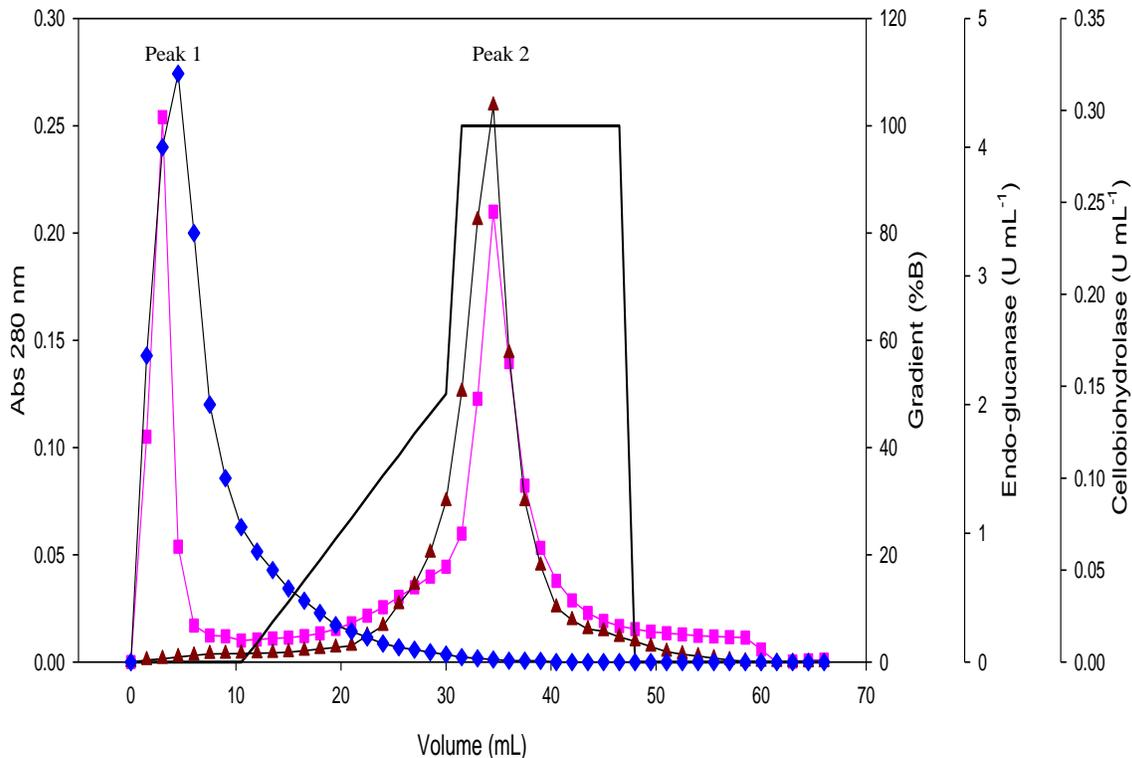
**Fig. 3.** Protein purification from the culture filtrate by hydrophobic chromatography using a HiTrap Phenyl FF column. (■) represents the distribution of the protein and elution profile of the proteins recorded at 280 nm; (—) gives profile of the 50 mM NaAc gradient on endoglucanases (▲) and cellobiohydrolase (◆)
