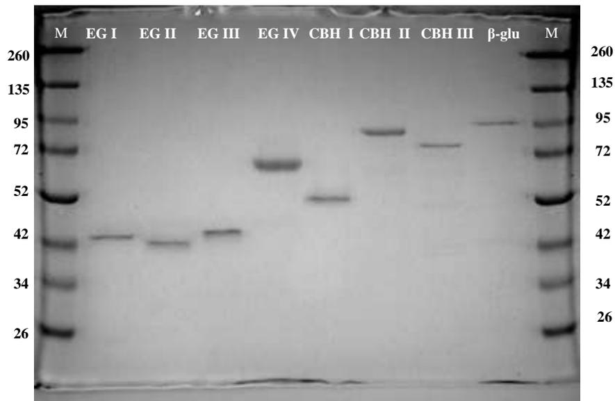
**Fig. 1.** Purification of cellulases from *A. terreus*. (a) The protein purification scheme from the culture filtrate. The parameters used in each purification step are described in Table 2. (b) SDS-PAGE (12% gel) of the purified enzymes (endoglucanases, cellobiohydrolase, and  $\beta$ -glucosidase)
