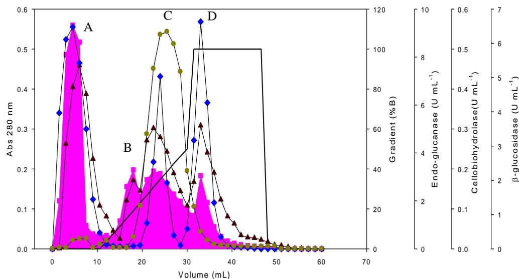
**Fig. 2.** Protein purification of the culture filtrate by anion exchange chromatography using a HiTrap QFF column. Distribution of the protein and elution profile of the proteins recorded at 280 nm (■); profile of the 1 M NaCl gradient (—) on endoglucanases (▲), cellobiohydrolase (◆), and β-glucosidase (●)
