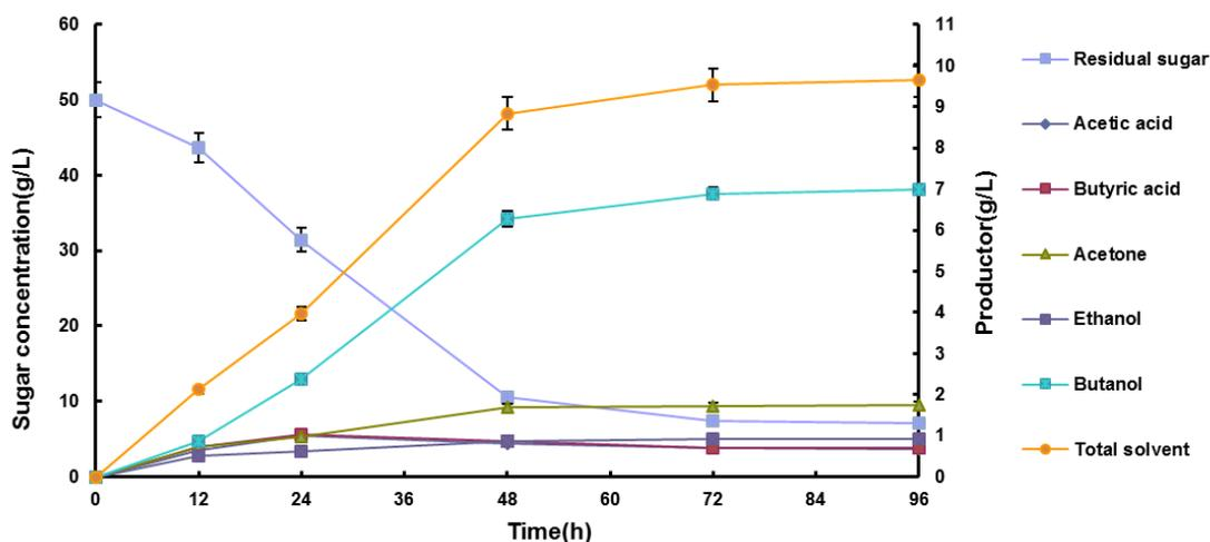
**Fig. 2.** Fermentation of poplar wood hydrolysates in the presence of other medium components (Second Mode). The figure shows the concentration of organic acids and solvents (acetone, butanol, ethanol) as a function of fermentation time.
