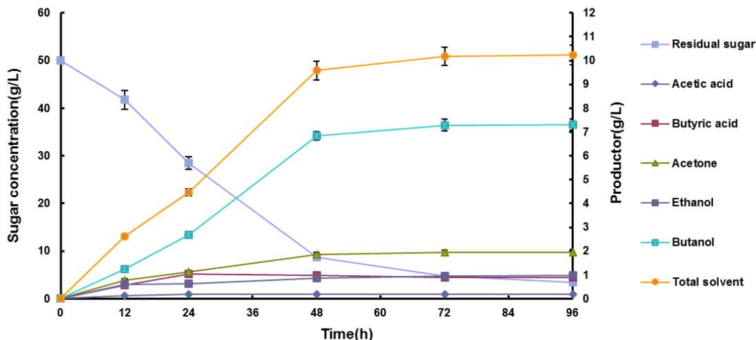
**Fig. 3.** Fermentation of poplar wood hydrolysates with additional mixed sugars (Third mode). The figure shows the concentration of organic acids and solvents (acetone, butanol, ethanol) as a function of fermentation time.
