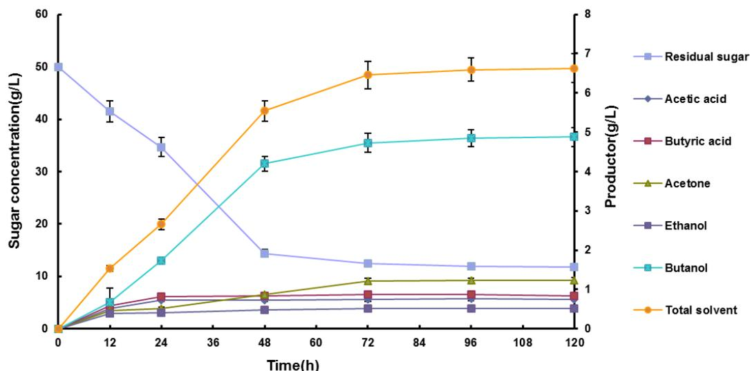
**Fig. 1.** Direct fermentation of poplar wood hydrolysates to biobutanol with no additives (First mode). The figure shows the concentration of organic acids and solvents (acetone, butanol, ethanol) as a function of fermentation time.
