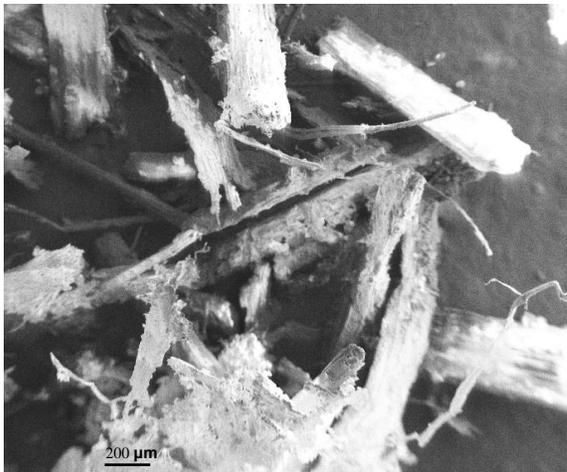
**Fig. 2b.** SEM image of MxG pretreated at 170 °C for 15 min
