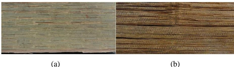
**Fig. 3.** The surface color of OBFM. (a): before heat treatment; (b): after heat treatment
