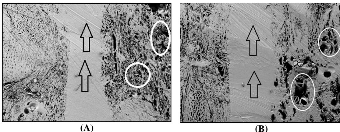
**Fig. 3.** SEM image of compressed OPT at 100  $\mu\text{m}$ , exposed to uncontrolled weather for 3 months: (A) laminated with 250  $\text{g}/\text{m}^2$  ASR sample, (B) laminated with 500  $\text{g}/\text{m}^2$  ASR sample (arrows show the glue line and circles show damaged parenchyma).
