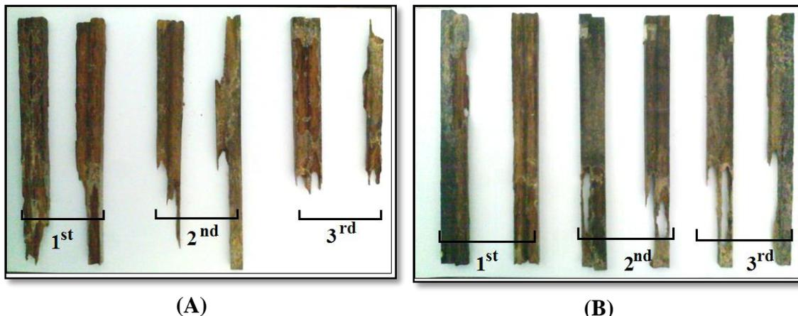
**Fig. 2.** Soil burial tests of compressed OPT samples retained after the 1<sup>st</sup>, 2<sup>nd</sup>, and 3<sup>rd</sup> months. (A) laminated with 250 g/m<sup>2</sup> spread rate PVAc, (B) laminated with 500 g/m<sup>2</sup> spread rate PVAc
