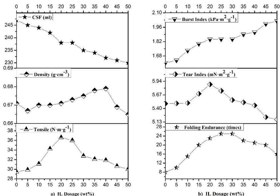
**Fig. 3.** Effect of IL dosage on the physical properties of the recycled fibers; pretreatment was conducted at a moisture content of 65% at 60 °C for 60 min
