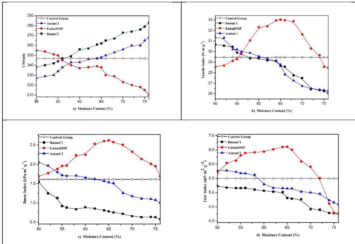
**Fig. 2.** Effect of moisture content on the physical properties of recycled fibers; the pretreatment was conducted at an IL concentration of 30 wt-% (based on oven-dried pulp) at 60 °C for 60 min
