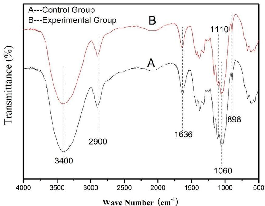
**Fig. 5.** FTIR spectra of (A) the control group and (B) the sample pretreated with [EMIM]DMP; pretreatment was conducted with a moisture content of 65% at 80 °C for 60 min at a dosage of 20 wt-%
