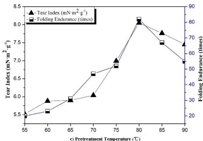
**Fig. 4.** Effect of temperature on physical properties; the pretreatment was conducted at a moisture content of 65% for 60 min with an [EMIM]DMP dosage of 20 wt-%
