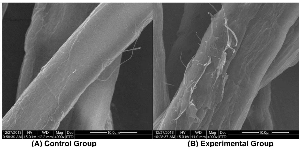
**Fig. 6.** SEM images of (A) the control group and (B) the sample pretreated with [EMIM]DMP; pretreatment was conducted with a moisture content of 65% at 80 °C for 60 min at a dosage of 20 wt-%
