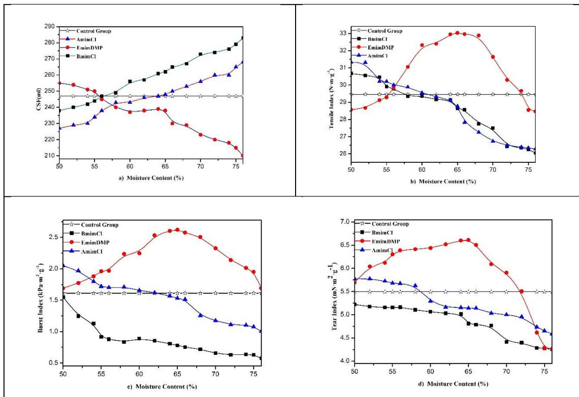
**Fig. 2.** Effect of moisture content on the physical properties of recycled fibers; the pretreatment was conducted at an IL concentration of 30 wt-% (based on oven-dried pulp) at 60 °C for 60 min
