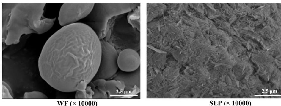
**Fig. 1.** SEM images of the WF and SEP
