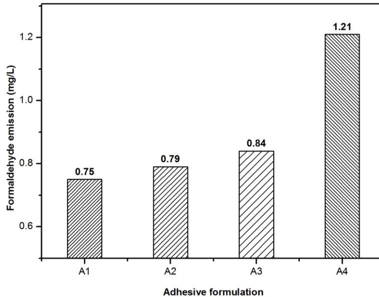
**Fig. 4.** The formaldehyde emissions of the plywood bonded by MUF resin with various filler formulations: (A1) 100% WF, (A2) 40% SEP + 60% WF, (A3) 80% SEP + 20% WF, and (A4) 100% SEP
