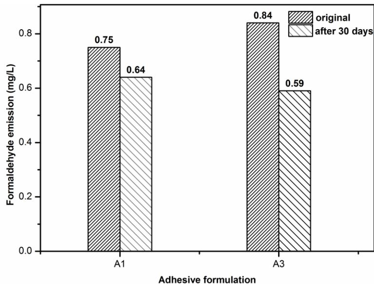
**Fig. 5.** Comparison of the initial formaldehyde emissions and the values after 30 days for plywood bonded by MUF resin with various filler formulations: (A1) 100% WF and (A3) 80% SEP + 20% WF
