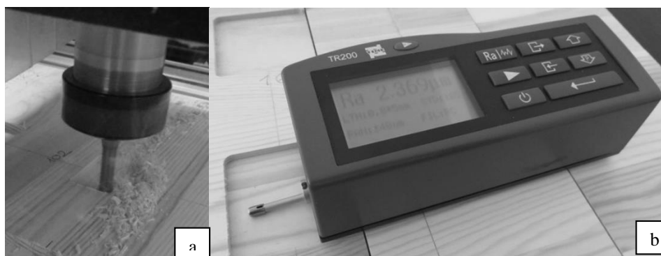
Fig. 1. (a) CNC milling machine during wood machining; (b) surface roughness tester TR200
