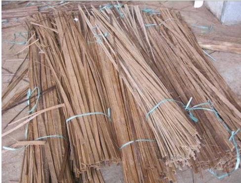
Fig. 1. Original bamboo strand bundles Fig. 2. Molds for parallel bamboo strand lumber
