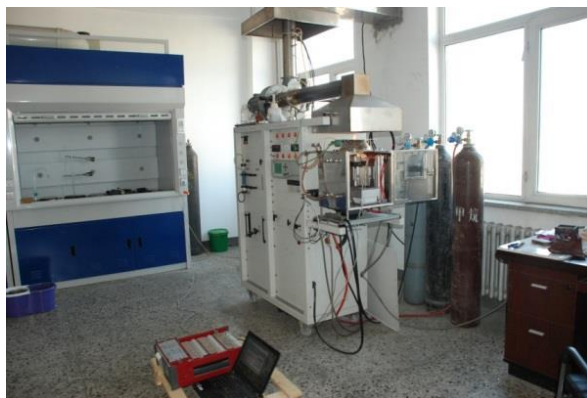
Fig. 2. The test apparatus: Cone calorimeter
