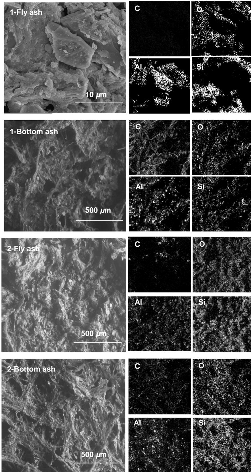
**Fig. 3.** The micromorphology and the elemental distribution of fly ash and bottom ash by SEM-EDS (Jeol JSM-6460). 1-fly ash that was tested by FEI Magellan-400. The labeling scheme, 1 and 2, denotes 500 mL or 900 mL Si-Al compounds, respectively.
