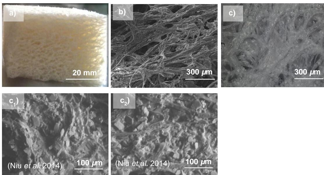
**Fig. 1.** The morphology of the ultra-low density fiberboards (ULDFs); a) the macromorphology of the ULDF without the Si-Al compound viewed using a common camera; b) the micromorphology of the ULDF without the Si-Al compounds from SEM; c) the micromorphology of the ULDF with the Si-Al compounds from an optical microscope; c<sub>1</sub>) and c<sub>2</sub>) show the micromorphology of the ULDF with 500 mL and 900 mL of Si-Al compounds from SEM, respectively.
