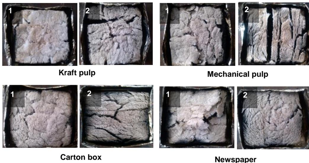
**Fig. 2.** The morphology of the burned ultra-low density fiberboards (ULDFs) by cone calorimetry at 780 °C. The labeling scheme, 1 and 2, represents the 500 mL or 900 mL amount of Si-Al compounds added, respectively. The size of each specimen was 100×100 mm before combustion.
