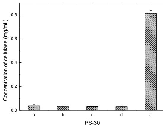
**Fig. 4.** The cellulase content of the permeate and retentate in the membrane separation process
