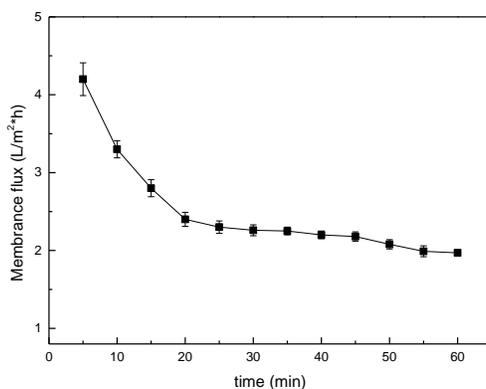
**Fig. 3.** The effect of the ultrafiltration time on membrane flux
