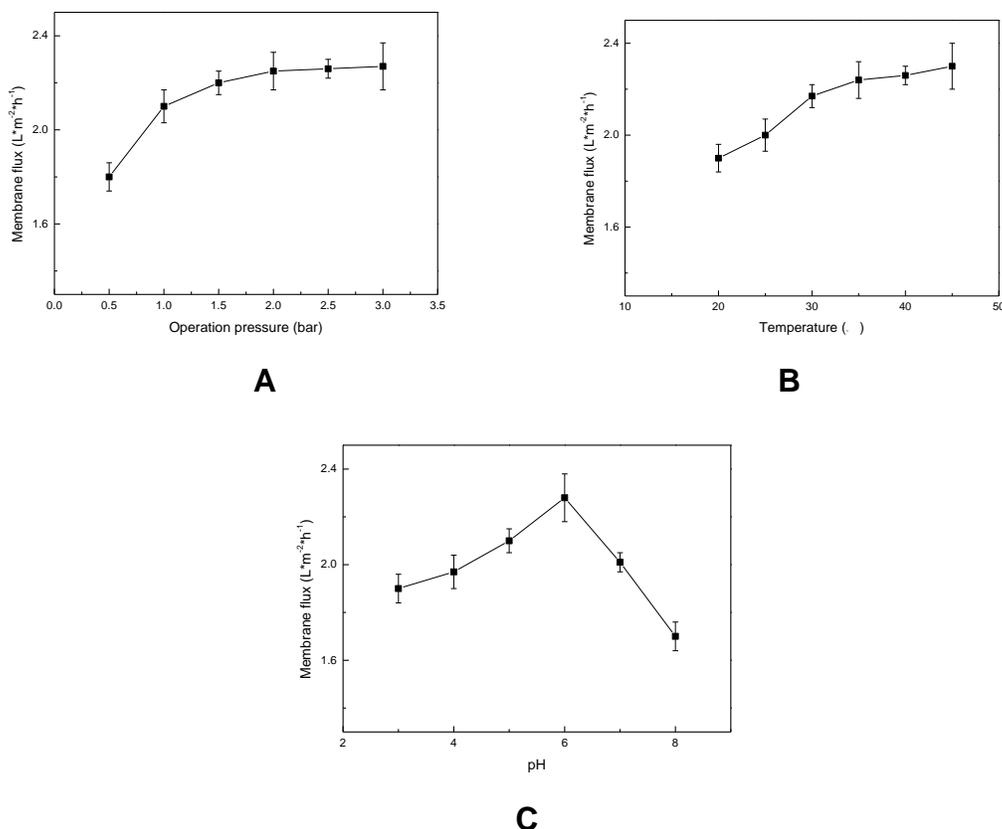
**Fig. 2.** Effect of different experimental parameters on membrane flux
