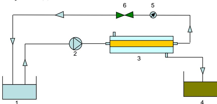
**Fig. 1.** Experimental set-up for membrane recovery system: 1. Hydrolysate; 2. peristaltic pump; 3. membrane module; 4. transdermal solution; 5 diaphragm; 6 relief valve
