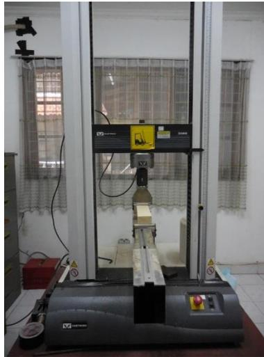
Fig. 2. MOR and MOE test using Universal Testing Machine
