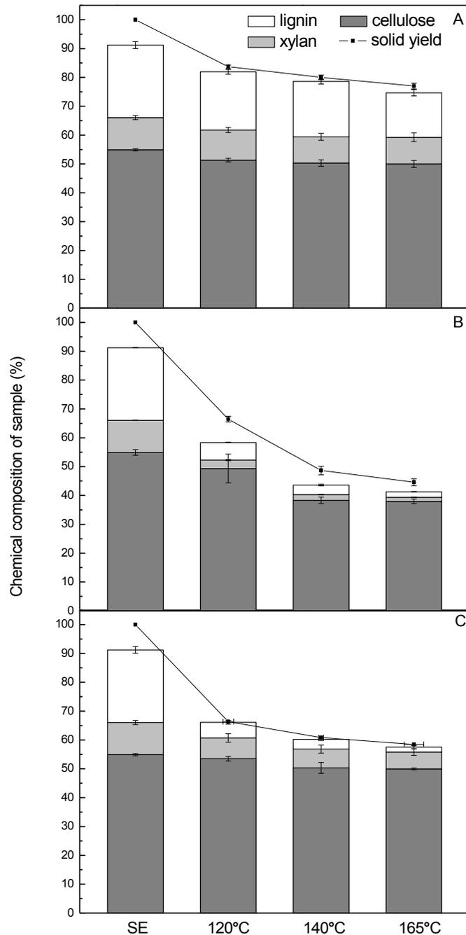
**Fig. 2.** A comparison of the chemical composition after the AS (A), AL (B), and ALS (C) pretreated bamboo samples
