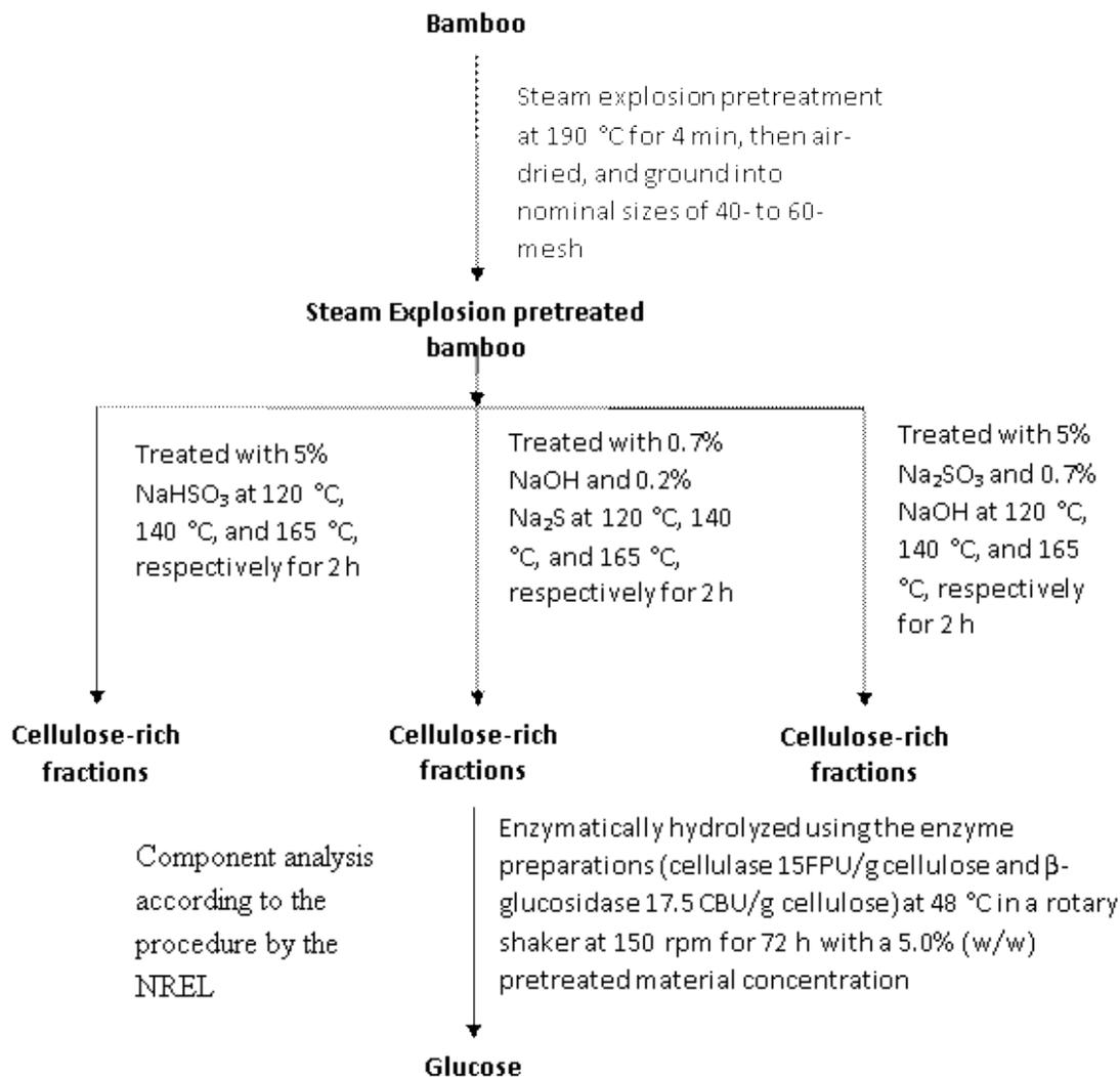
**Fig. 1.** Schematic showing the treatment of bamboo samples with the combination of steam explosion pretreatment and chemical pretreatments
