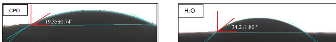
**Fig. 4.** Contact angles of CPO and H<sub>2</sub>O with POME at equilibrium
