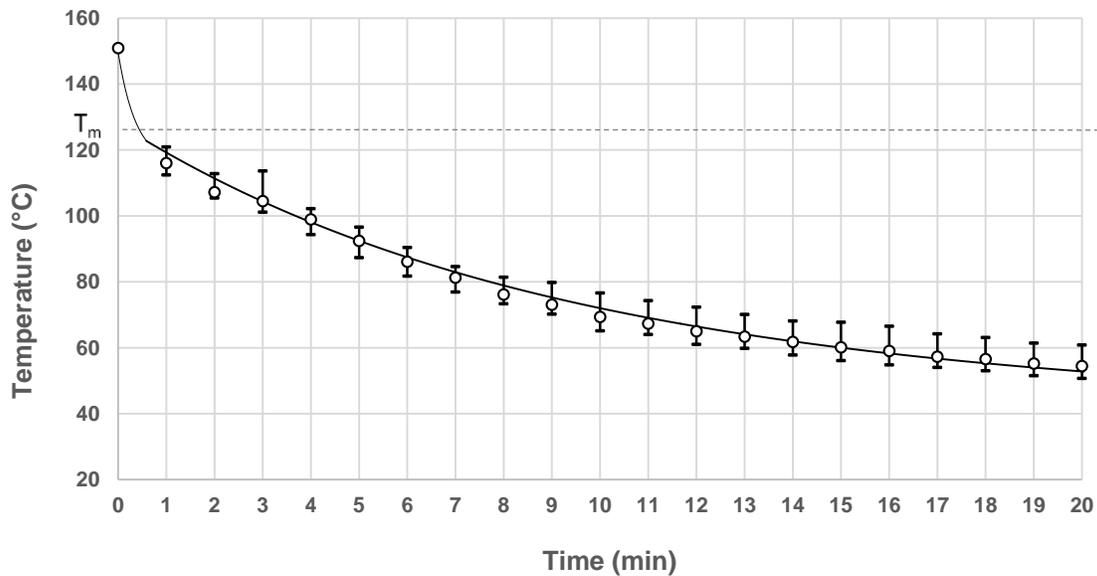
**Fig. 6.** Measured cooling and an overlaid curve fit with the bandwidth of the measurement indicated
