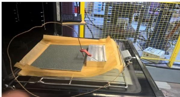
**Fig. 1.** Heat sensor attached and temperature measured from the edge of a WPC sheet
