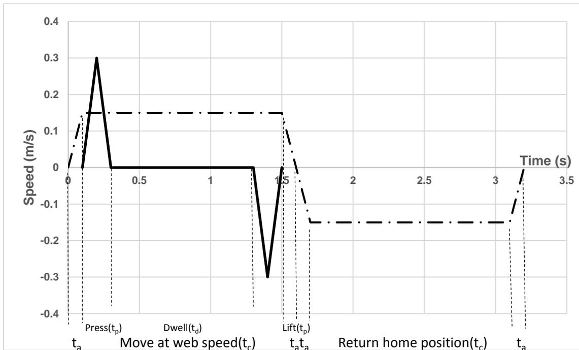
Fig. 10. Structure of KompoLine press cycle with time segments listed
