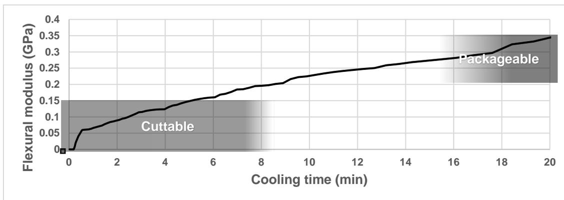
**Fig. 9.** Flexural modulus vs. cooling time overlaid by manufacturing slots
