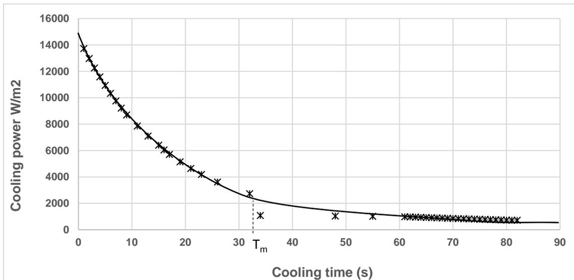
**Fig. 12.** Calculated cooling power in  $\text{W/m}^2$ , calculated using the heat capacity of HDPE and the measured cooling rate of the composite material.  $T_m$  indicates the melting point of the material.
