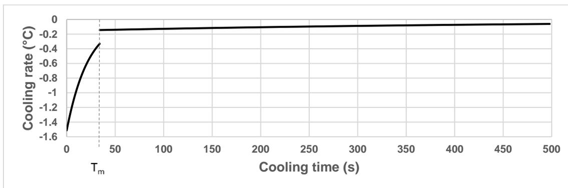
**Fig. 7.** Calculated cooling rates. The gap between the cooling rates at the melt temperature ( $T_m$ ) is caused by the curve fit approximation and is not an actual phenomenon.
