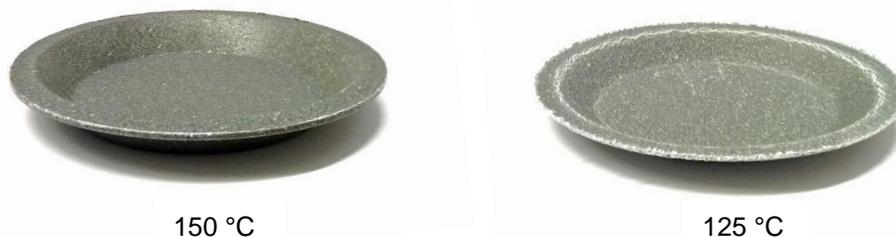
**Fig. 2.** The effects of temperature on product quality. The test specimens were heated from 150 and 125 °C before pressing. At 125 °C, visible cracks were observed and the surface finish was rough in comparison to the specimen at 150 °C.
