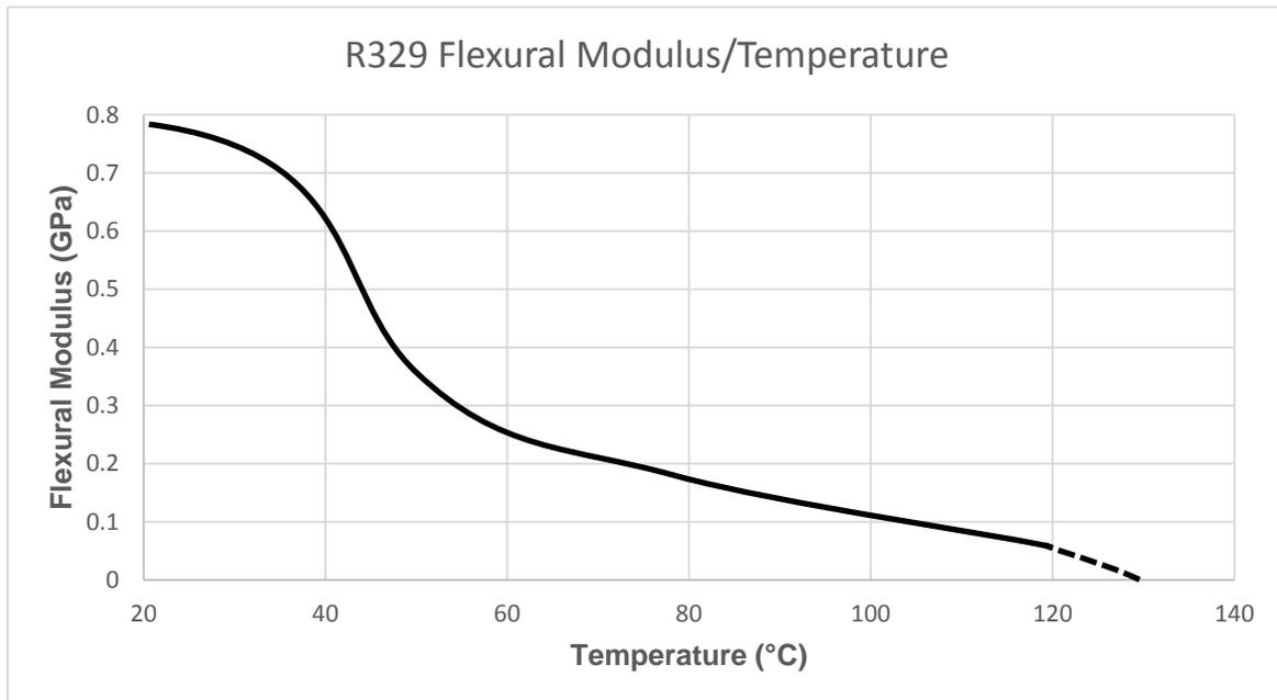
**Fig. 3.** Measured flexural modulus of the composite material in terms of temperature. The dashed line represents the temperature where the material started to have significant creep behavior, extrapolated from the measured results.
