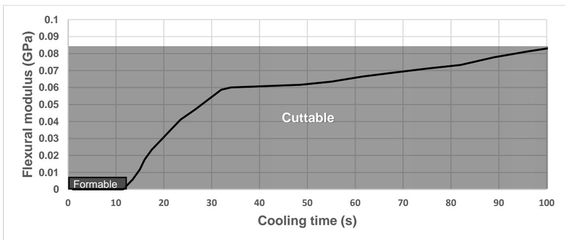
Fig. 8. Flexural modulus vs. cooling time overlaid by manufacturing slots
