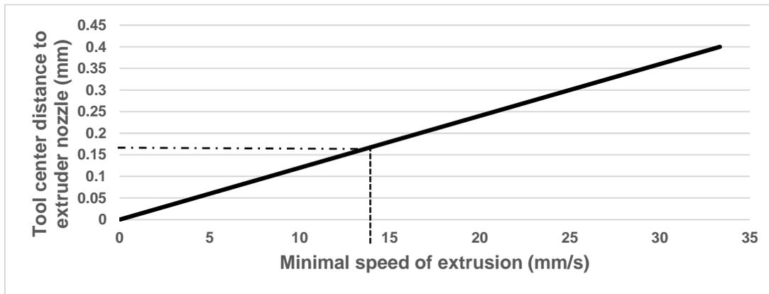
**Fig. 11.** Relationship between tool center distance to the nozzle and minimal speed of extrusion. Minimal feed time for LUT KompoLine with 350-mm tool width is highlighted.
