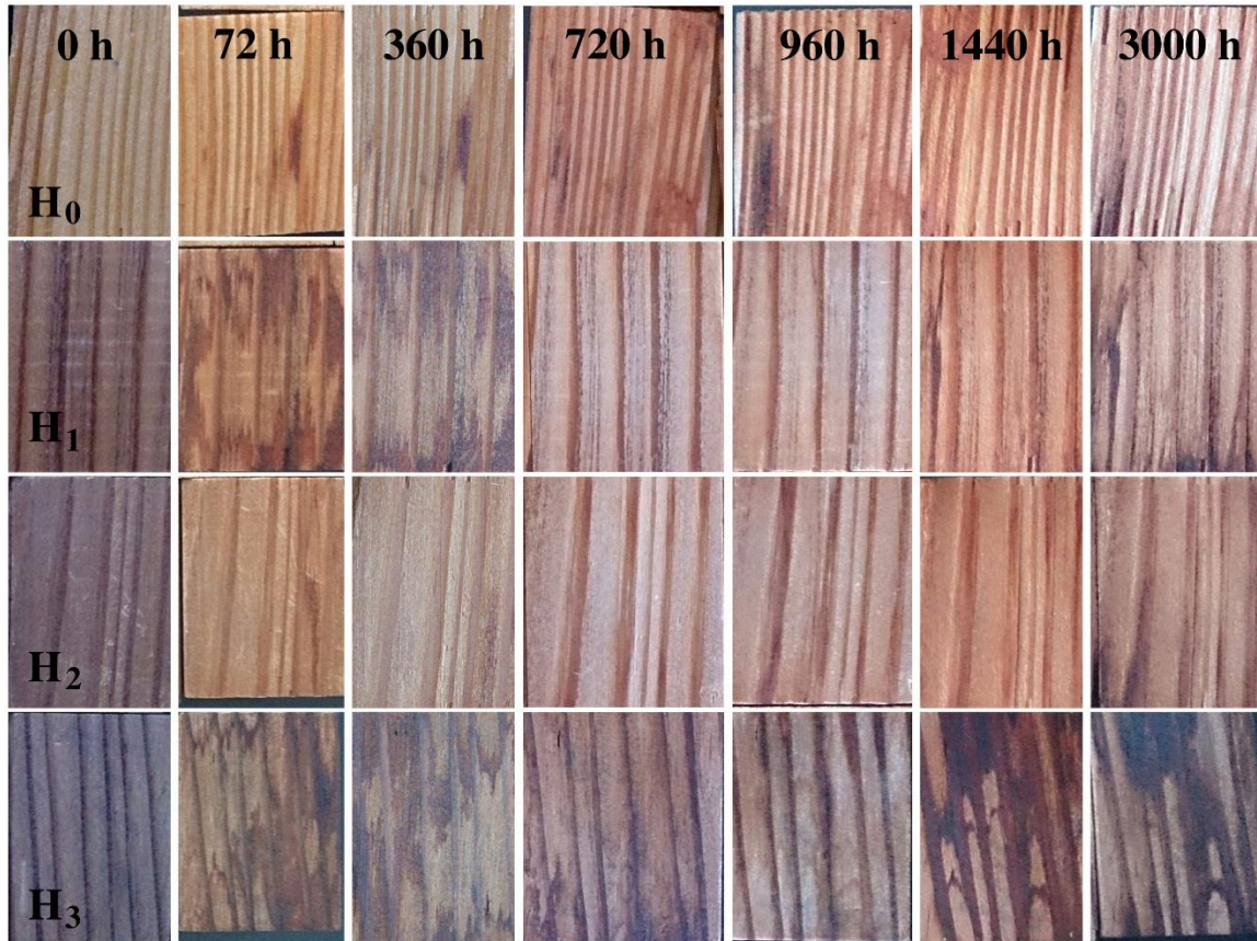
Fig. 1. The visual observation of heat-treated and untreated Larix spp. surfaces during different artificial weathering periods
