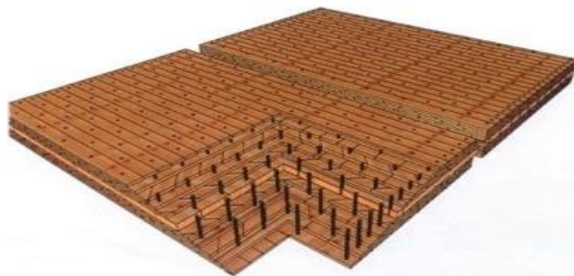
Fig. 5. Vertical dowelled system (Holz100) (Thoma 2000)
