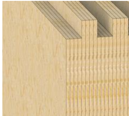
Fig. 3. Magnum board manufactured by bonded 25-mm OSB
