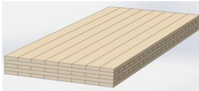
Fig. 2. Cross-laminated timber (CLT) panels
