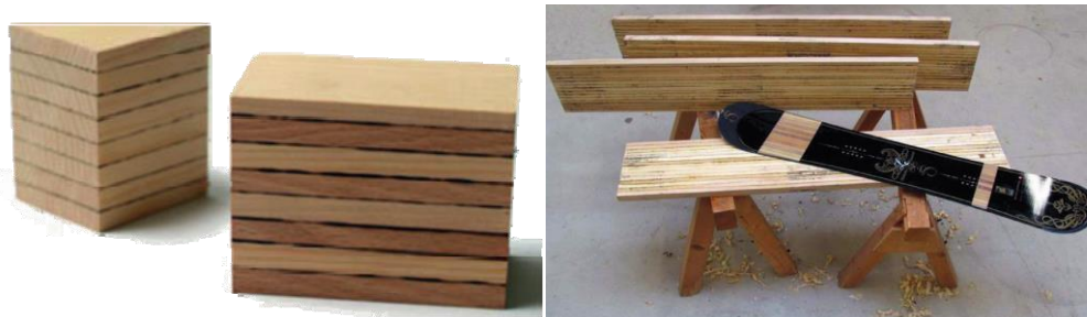
Fig. 9. Examples of wood welding (Vaziri 2011)
