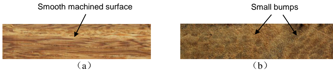
Fig. 6. Machined surface of bamboo scrimber during (a) longitudinal milling and (b) end-grain milling
