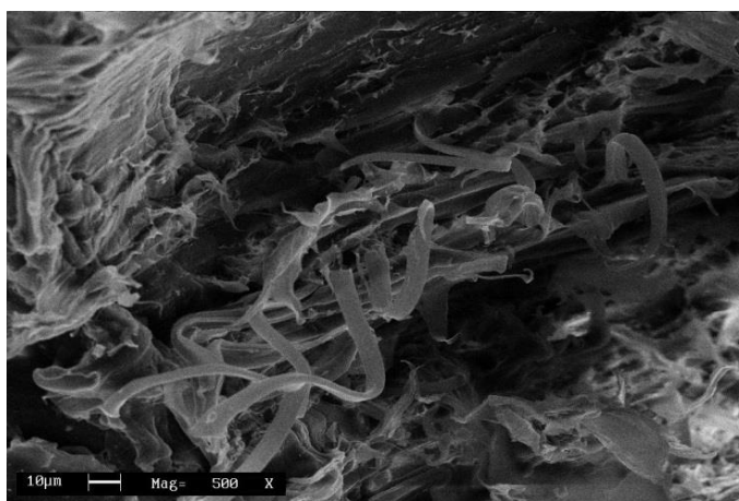
Fig. 8. SEM micrographs from vPP+nsWF composites
