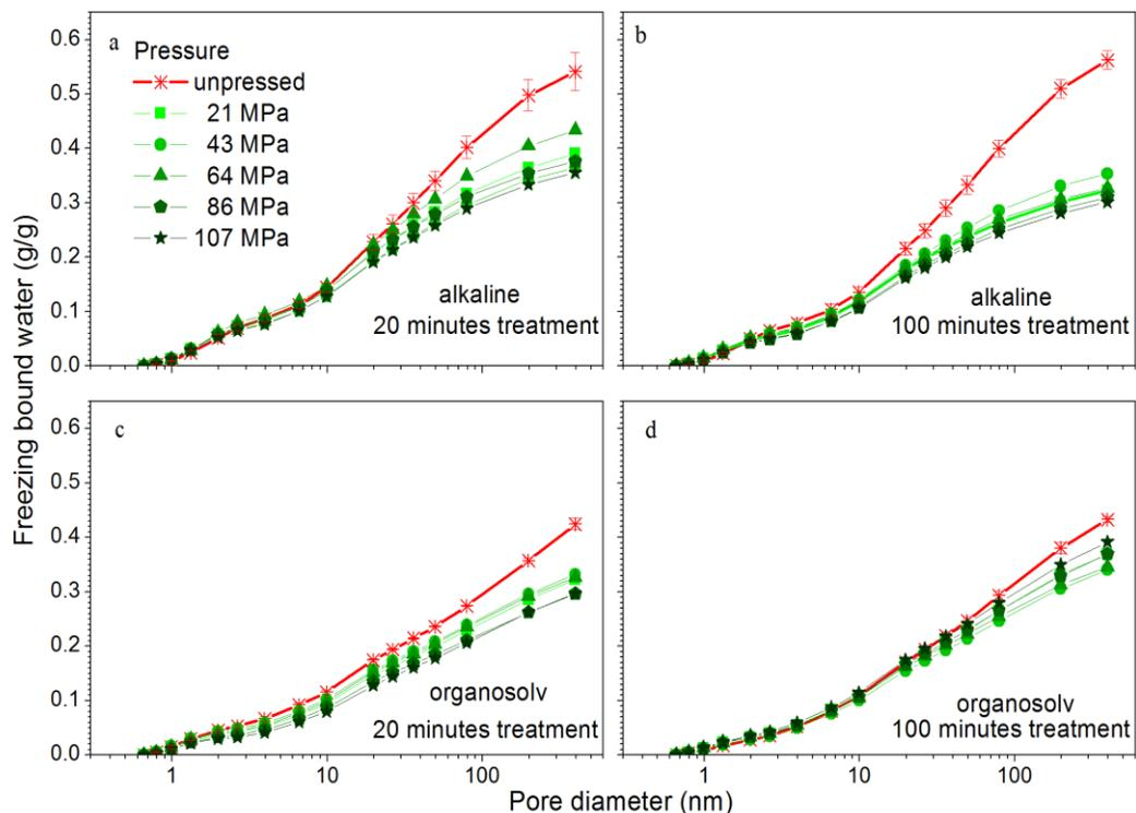
**Fig. 4.** Results of thermoporometry for alkaline (a and b) and organosolv (c and d) pulps, produced with 20 min (a and c) and 100 min (b and d) pulping times, before and after wet pressing at different pressures
