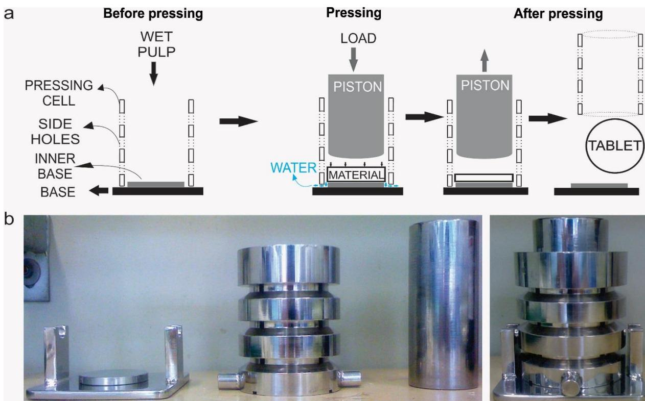
**Fig. 1.** System used for wet pressing: a) Sketch of a wet pressing test, b) Images of the disassembled (left) and assembled (right) compression cell
