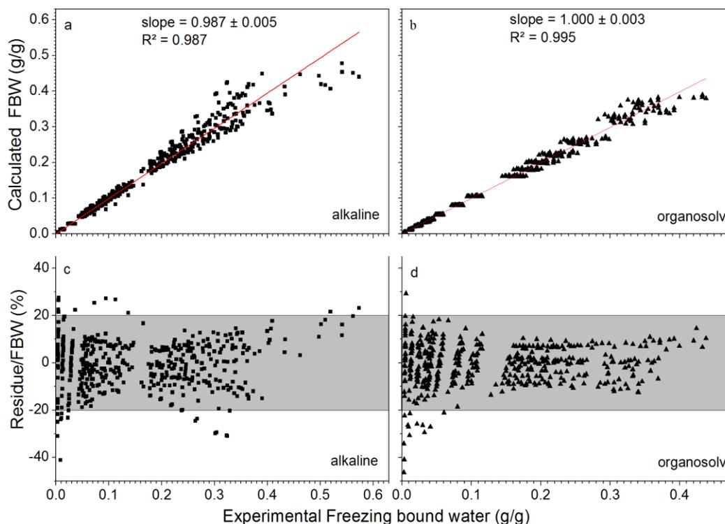
**Fig. 5.** Validation of linear regression of thermoporometry profiles for alkaline (a and c) and organosolv pulps (b and d)
