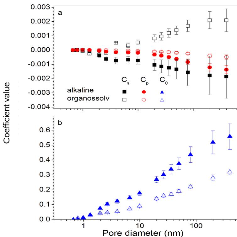
**Fig. 6.** Coefficients from linear regression of thermoporometry data of pressed pulps. Solubilization and pressure coefficients ( $C_s$  and  $C_p$ , respectively) are shown in a, while the coefficient  $C_0$  is shown in b. The coefficients  $C_s$ ,  $C_p$ , and  $C_0$  are calculated for every pore diameter recorded in the thermoporometry profiles
