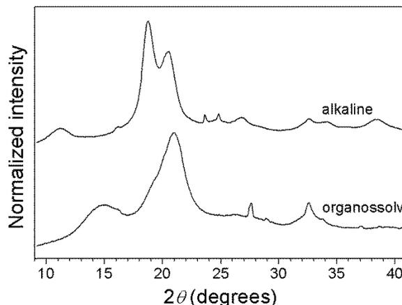
**Fig. 2.** Diffractograms of pulps produced by alkaline and organosolv treatments (reaction time of 60 min), showing the typical patterns of cellulose II and cellulose I, respectively
