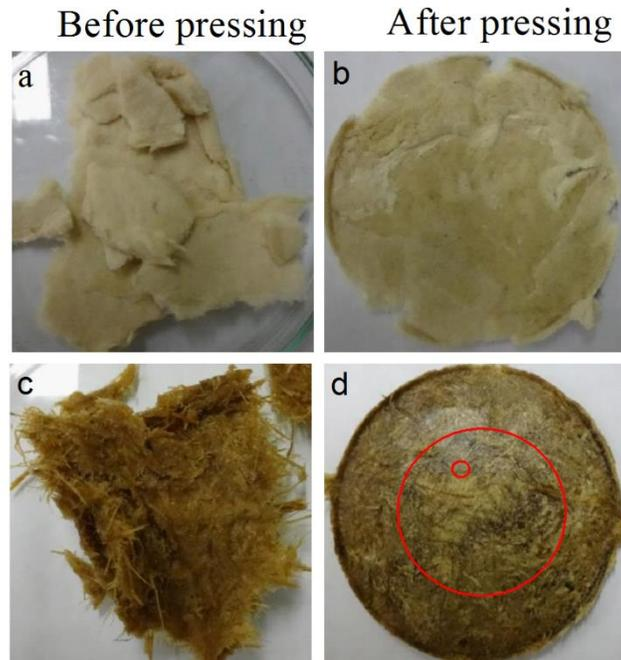
**Fig. 3.** Images taken of alkaline (a and b) and organosolv (c and d) pulps before and after wet pressing. The materials shown in the images were pulped for 20 min and pressed at 107 MPa. The circles in (d) have diameters of 3 cm and 3 mm, respectively, corresponding to the region considered for sampling and the actual size of one sample selected for thermoporometry analysis
