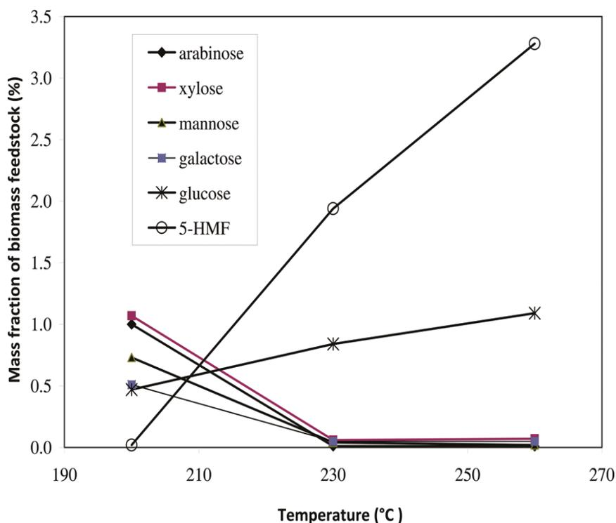
**Fig. 2.** Composition of precipitates in the aqueous output stream from loblolly pine wet torrefaction at various temperatures. Each mass fraction is reported as a fraction of the dry biomass feed (Yan *et al.* 2010).
