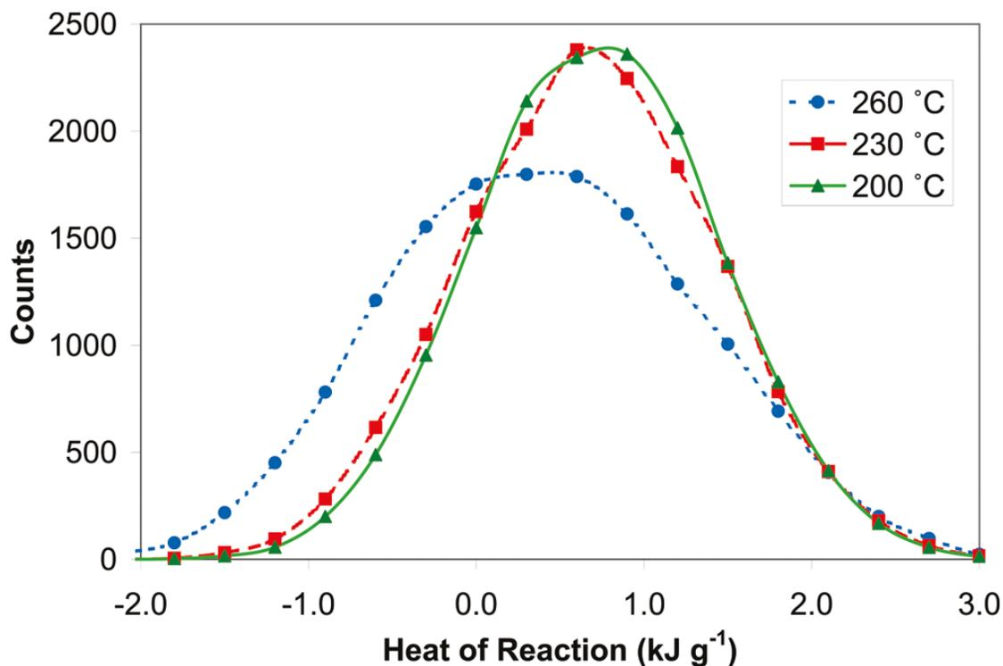
**Fig. 3.** Frequency distributions of the heats of reaction, during wet torrefaction of loblolly pine at three temperatures (Yan *et al.* 2010)
