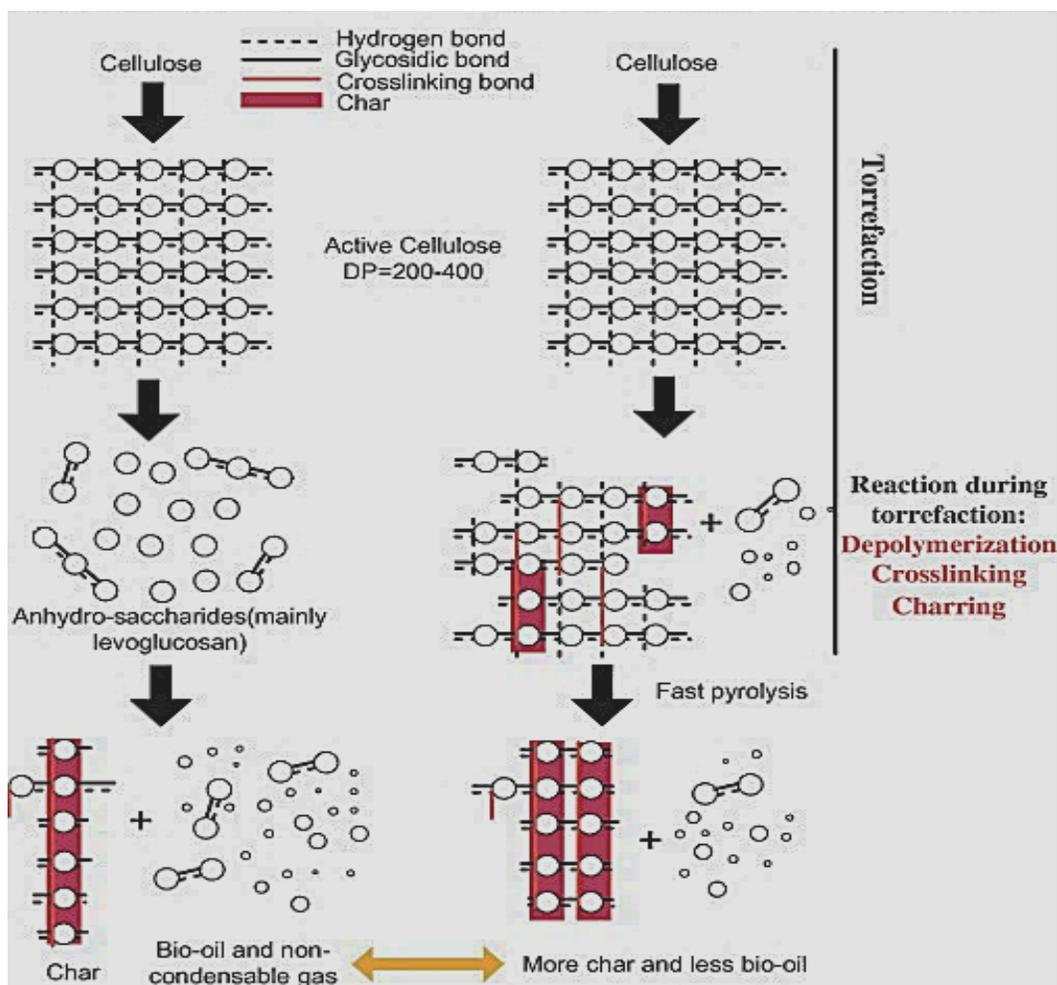
**Fig. 6.** Effects of torrefaction on the fast pyrolytic decomposition of cellulose (Chaiwat *et al.* 2008). Figures used by permission of copyright holder.
