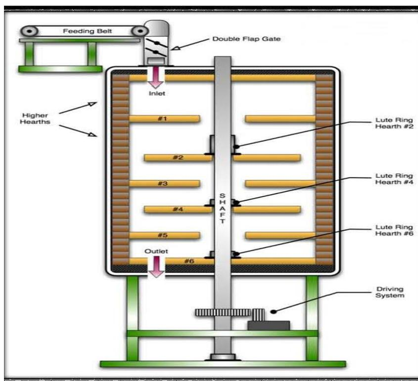
Fig. 10b. Schematics of a multiple hearth furnace
