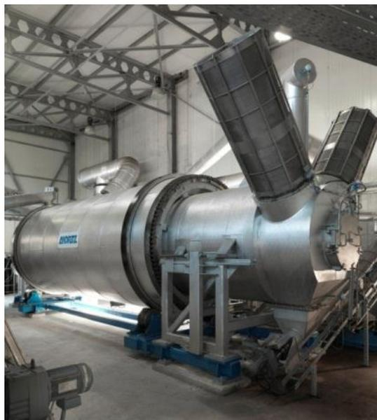
Fig. 8a. Rotary drum reactor (Thamer 2013)
