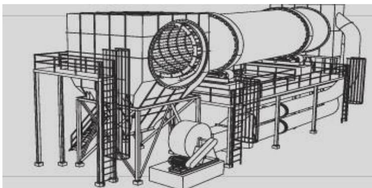
Fig. 8b. Schematics of a rotary drum reactor
