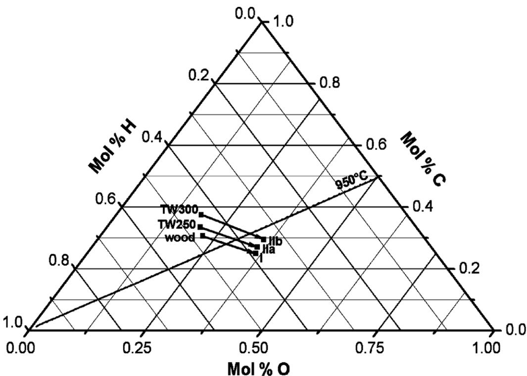
Fig. 4. CHO diagram illustrating gasification of wood and torrefied wood (TW), where the torrefied wood was produced at 250 and 300 °C, then gasified at 950 °C (Prins *et al.* 2006a)
