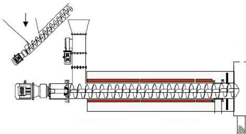
Fig. 9b. Schematics of a screw reactor
