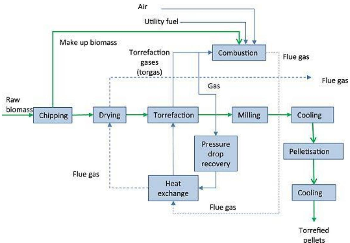
Fig. 1. Overview of an integrated torrefaction plant (Kiel *et al.* 2012)
