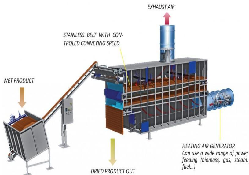
**Fig. 14.** Schematics of a belt dryer ([www.biogreen-energy.com](http://www.biogreen-energy.com))
