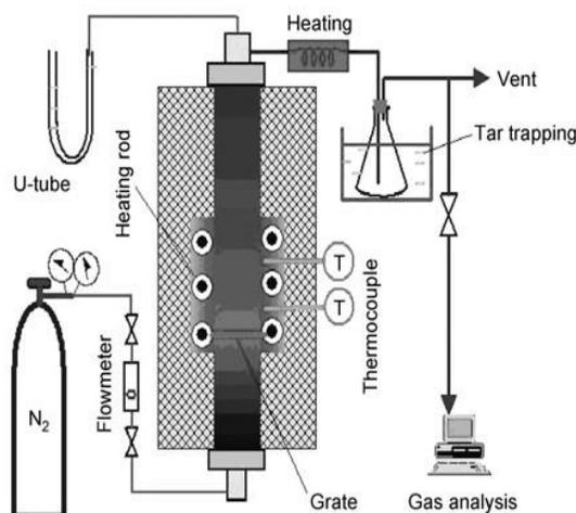
Fig. 7b. Schematics of a fixed bed reactor
