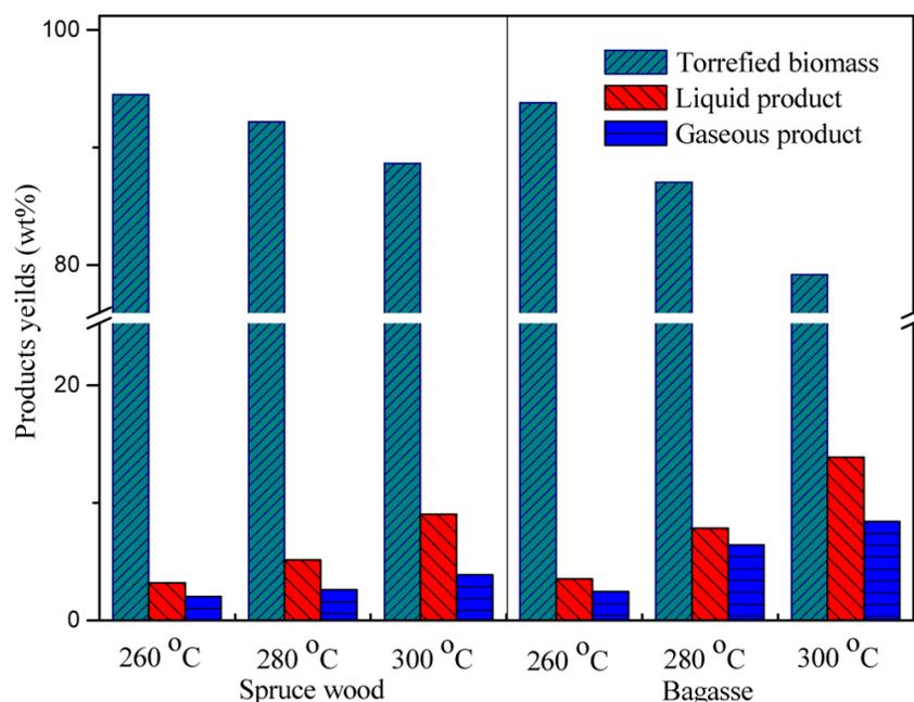
**Fig. 5.** Effect of torrefaction temperature on the distributions of biomass torrefaction product phases (Chang *et al.* 2012)
