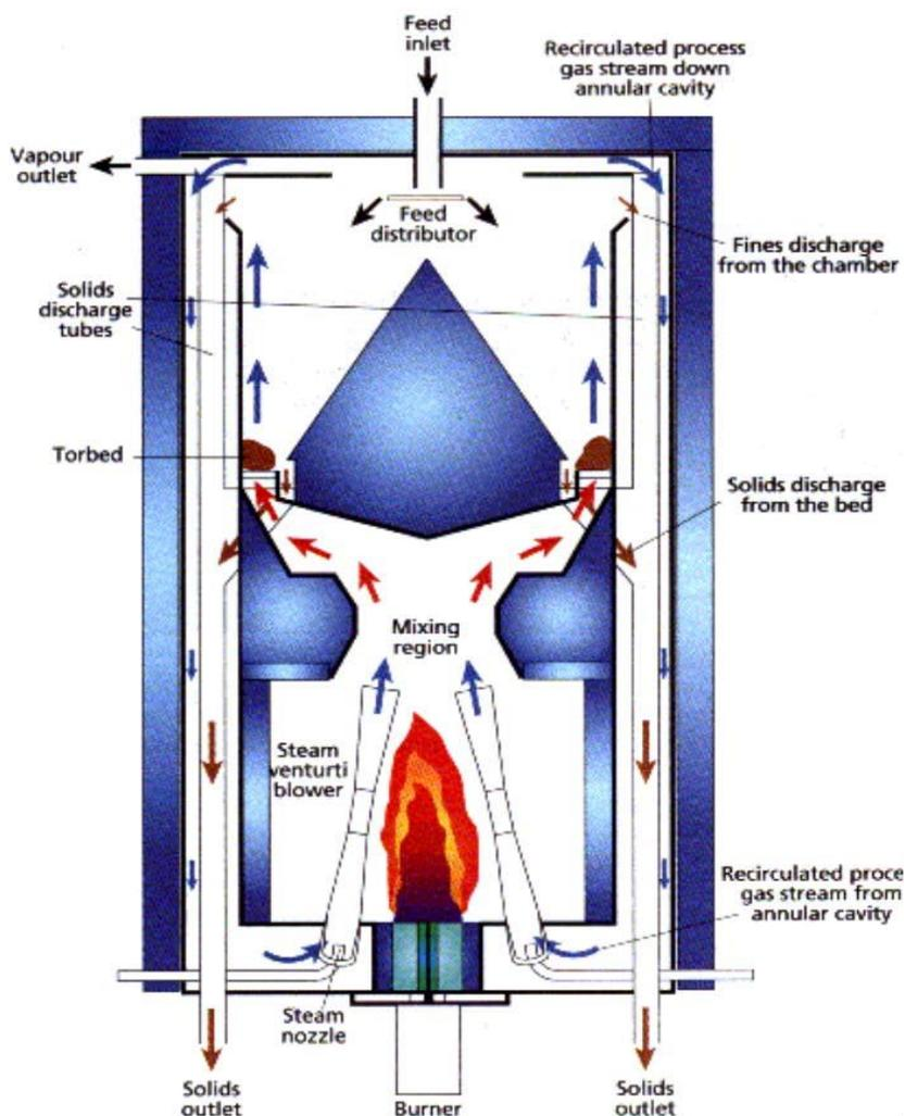
Fig. 11b. Schematics of a torbed reactor
