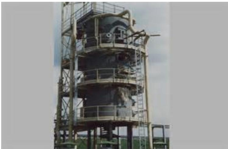
Fig. 10a. Multiple hearth furnace (fgcgroupllc.com)
