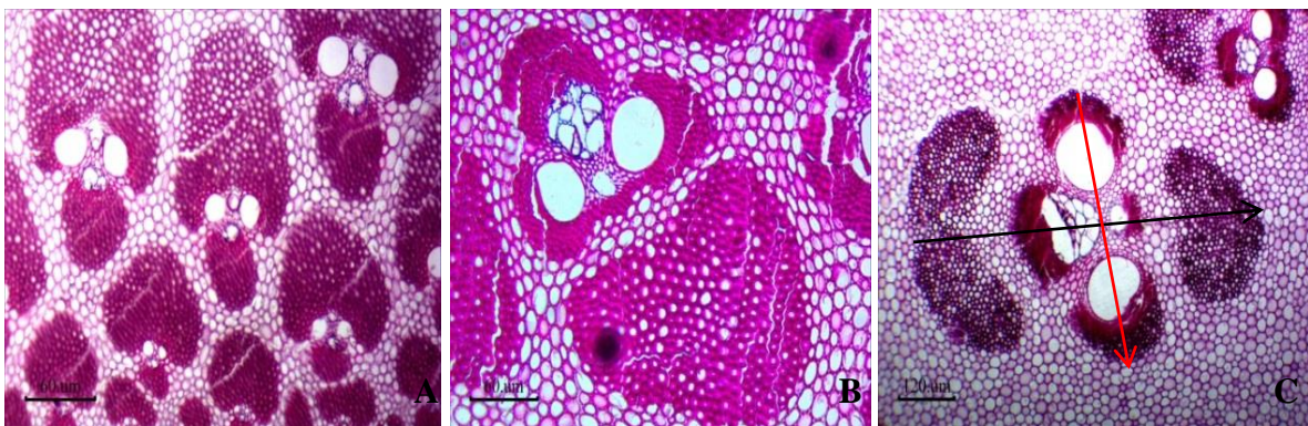
Fig. 1. The vascular bundle types of D. brandisii in transverse section: A, semi-undifferentiated type in outer zone; B, broken-waist type in middle zone; and C, double broken-waist type in inner zone. The black and red arrows represent the radial length and tangential diameter of vascular bundles, respectively.
