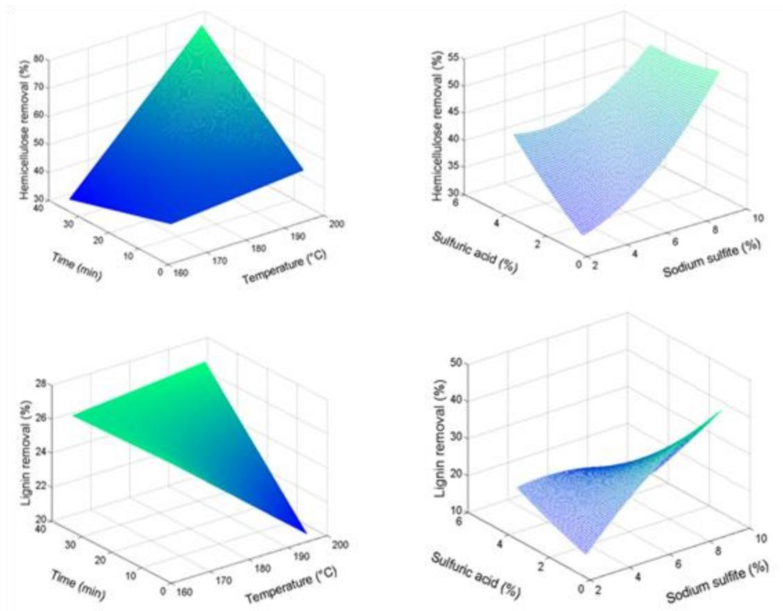
**Fig. 1.** Effects of pretreatment conditions on lignin and hemicellulose removals during sulfite pretreatment of manure
