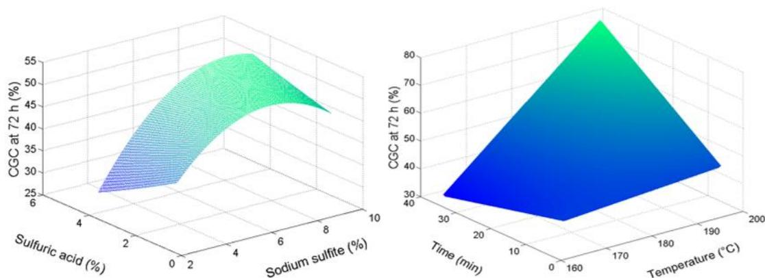
**Fig. 4.** Effects of pretreatment conditions on cellulose-to-glucose conversion (CGC) after 72 h in sulfite-pretreated manure
