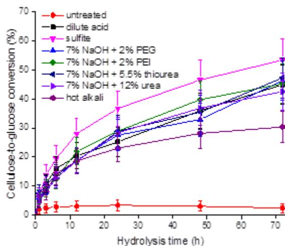
**Fig. 6.** Time-dependent enzymatic hydrolysis profiles of manure pretreated by sulfite, diluted acid, and alkali
