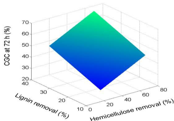
**Fig. 3.** Effects of lignin or hemicellulose removal on cellulose-to-glucose conversion (CGC) after 72 h in sulfite-pretreated manure
