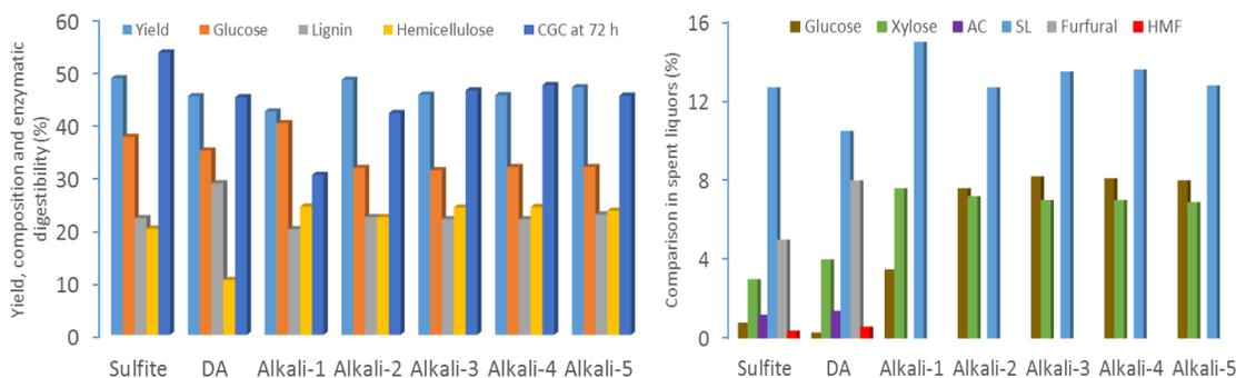
**Fig. 5.** Comparison of sulfite, dilute acid, and alkali pretreatments of manure
