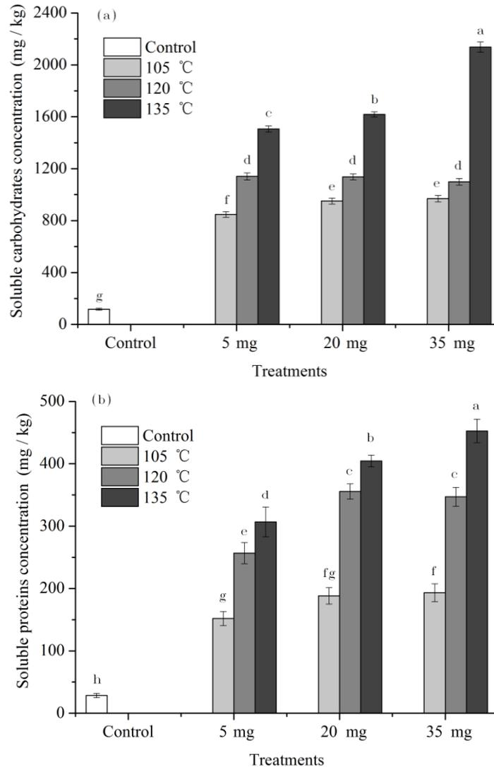
**Fig. 1.** Concentrations of the soluble carbohydrates (a) and proteins (b) in the DAS after thermal-alkaline pretreatment. Bars indicate the standard deviation (SD). Note: The letters (a, b, c.....) behind the data represent the significant difference ( $p < 0.05$ ) among different groups.
