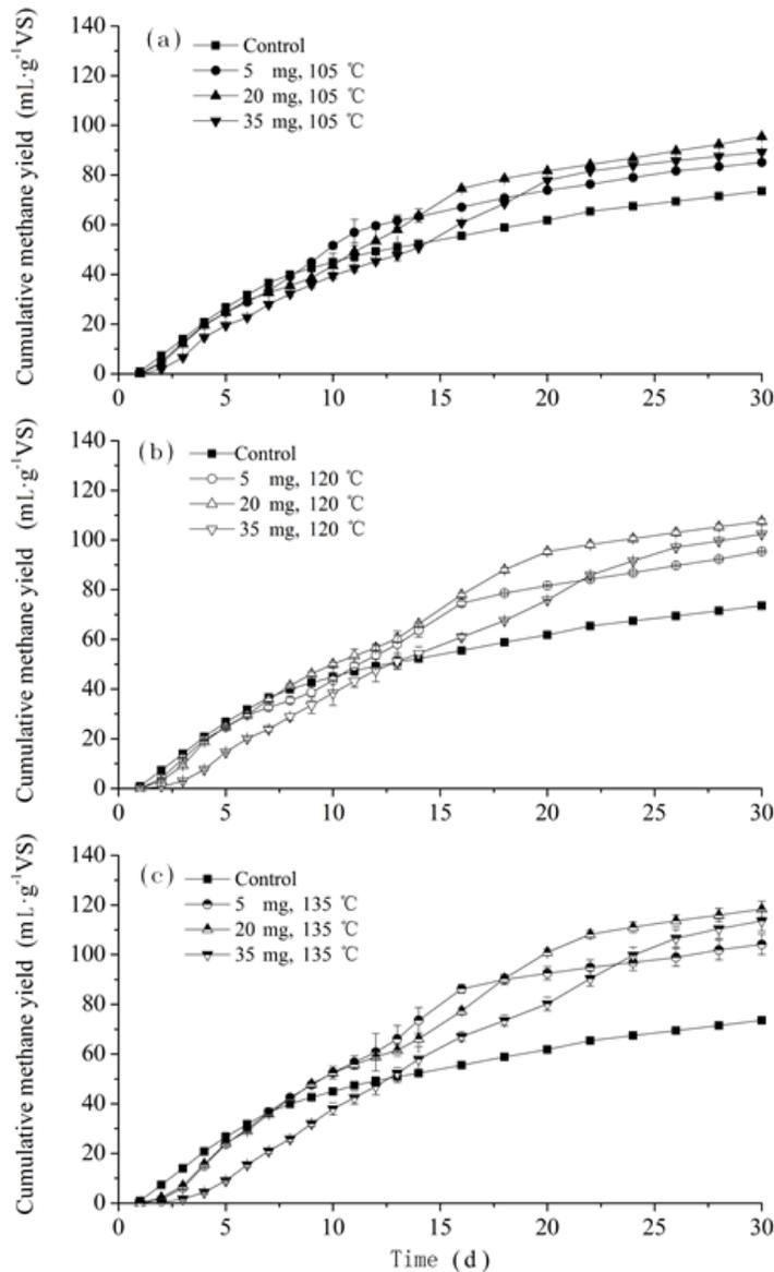
**Fig. 3.** Cumulative methane yield during high-solid anaerobic digestion after thermal-alkaline pretreatment
