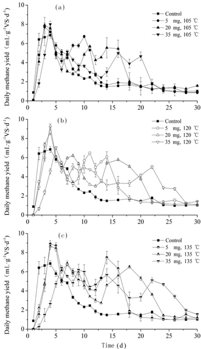
**Fig. 2.** Daily methane yield during high-solid anaerobic digestion after thermal-alkaline pretreatment
