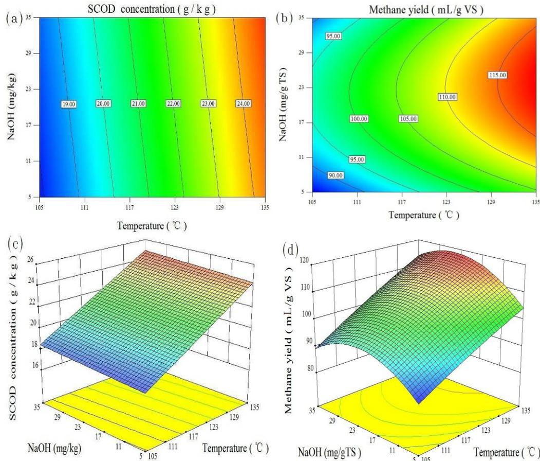
**Fig. 4.** Contour and 3D response surface plots: interactive effects of temperature and alkaline dose on SCOD concentration and methane yield
