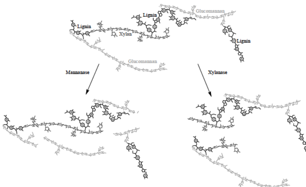
Fig. 2. Schematic presentation of how selective hemicellulases affect a “mixed” hemicellulose/lignin molecule. A selective enzyme attacking one hemicellulose affects the entire molecule and thereby also influences the solubility and extractability of lignin and other polysaccharides.
