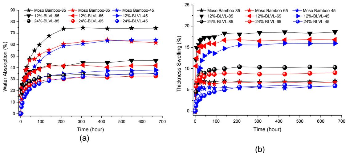
**Fig. 1.** Durability of moso bamboo strips and BLVLs: (a) the effect of temperature on the water absorption process for moso bamboo strips and BLVLs and (b) the effect of temperature on the thickness swelling rate for moso bamboo strips and BLVLs
