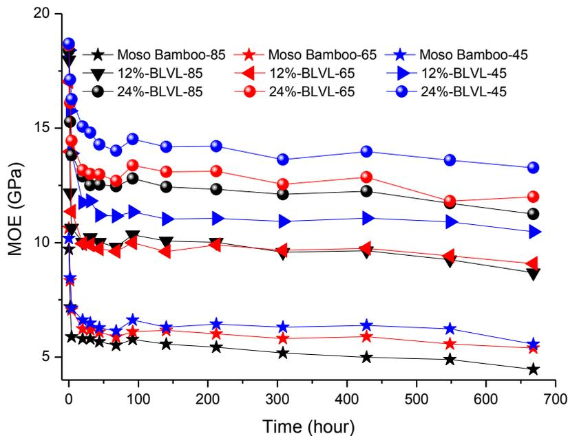
Fig. 3. The effect of temperature on the MOE for moso bamboo strips and BLVL samples
