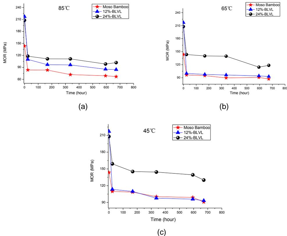
**Fig. 4.** The effect of temperature on the MOR for moso bamboo strips and BLVL samples
