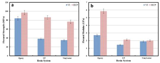
Fig. 3. Comparison of (a) Flexural strength, (b) Flexural moduli for composites using VI and HCP methods
