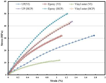
Fig. 2. Stress–strain curves of polymer reinforced kenaf fiber composites using HCP and VI methods.
