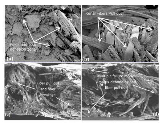
**Fig. 6.** SEM images of tensile section failure of kenaf reinforced UP composites (a) and (b) using VI method (c) and (d) using HCP method
