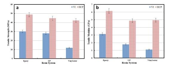
Fig. 1. Comparison of (a) Tensile strength, (b) Tensile moduli for composites using VI and HCP methods
