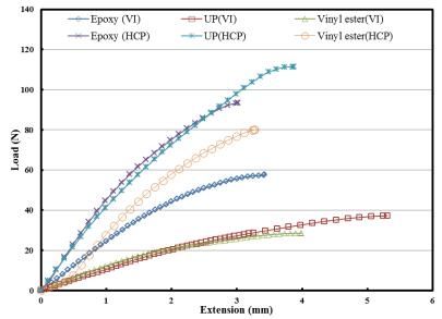
**Fig. 4.** Flexural load–extension relationship of kenaf fiber composites using different polymers types and methods
