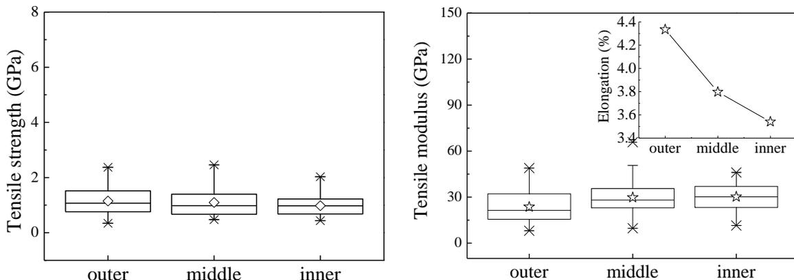
**Fig. 7.** Trends of tensile properties of bamboo fibres along the radius
