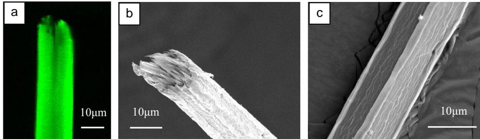
**Fig. 2.** Fracture surface under CLSM (a) and under FESEM (b), and the morphology (c) of single bamboo fibre
