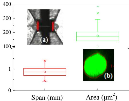
**Fig. 3.** Tensile span (a) and cross-sectional area (b) of a single bamboo fibre
