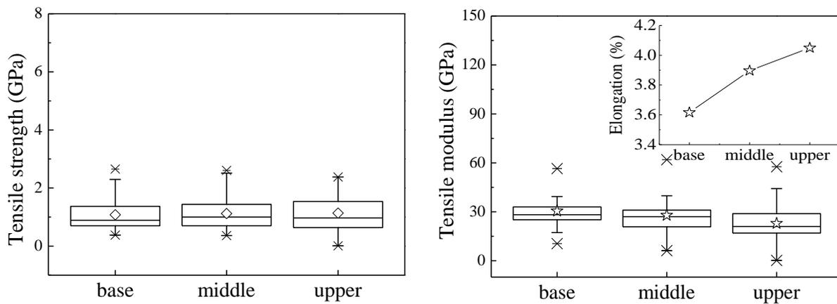
**Fig. 6.** Trends of tensile properties of bamboo fibres along culm height
