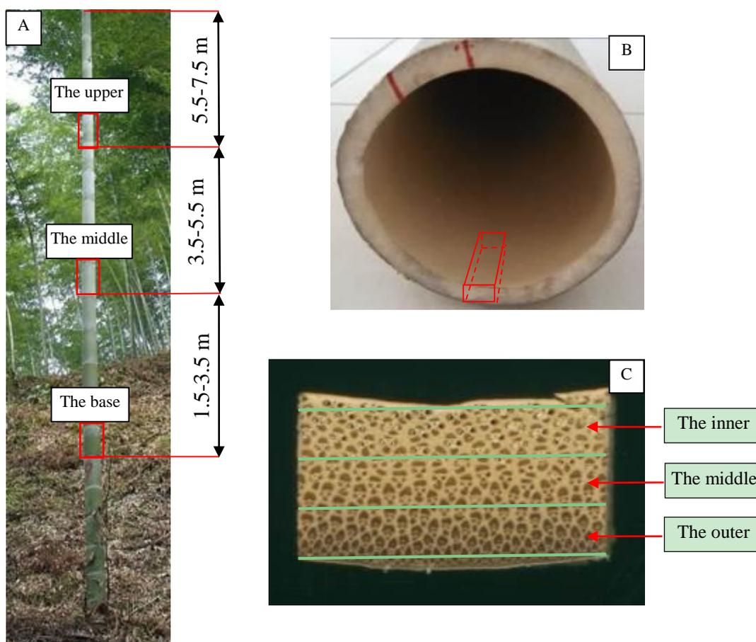
**Fig. 1.** The methods of splitting *D. farinosus* bamboo blocks (A and B) along different culm height positions and (C) along radial direction
