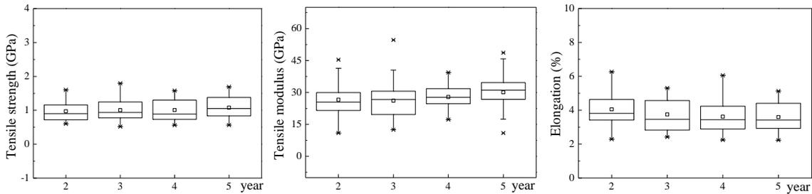
**Fig. 5.** Trends of tensile properties of single fibre with bamboo age
