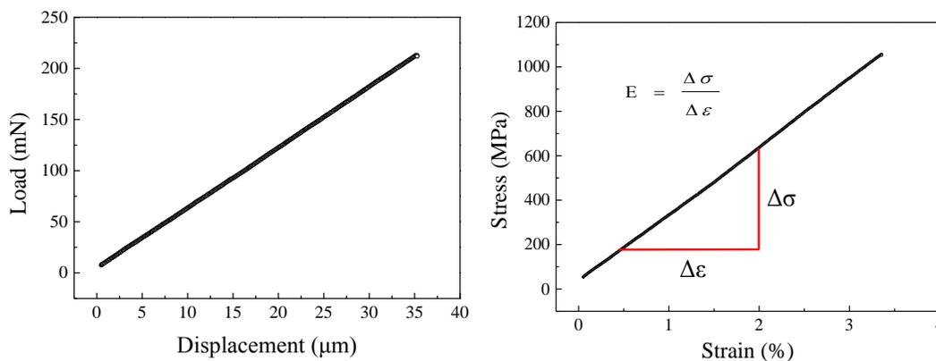
**Fig. 4.** Load-displacement and stress-strain curves
