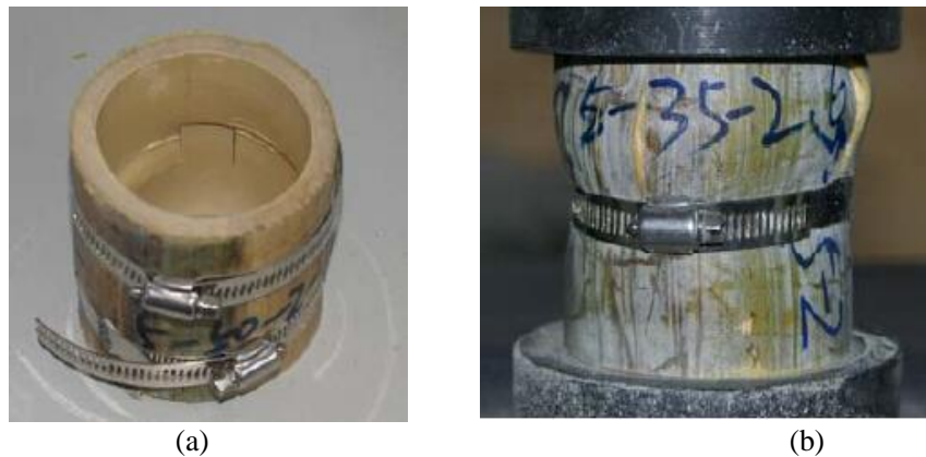
Fig. 4. Bamboo culm with hose clamps (a) before and (b) after compressive failure
