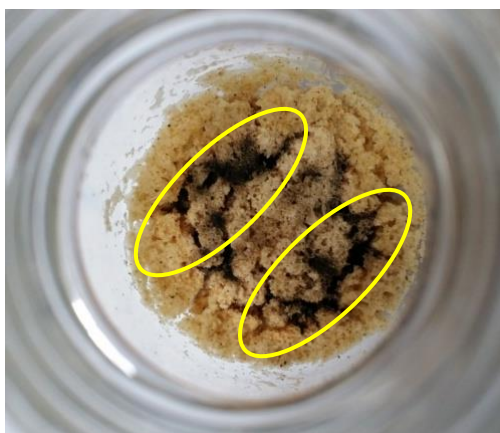
Fig. 1. Charring of pretreated SW (circled) at pretreatment conditions of 500 W microwave power, 3 min pretreatment duration, and 23% solid loading
