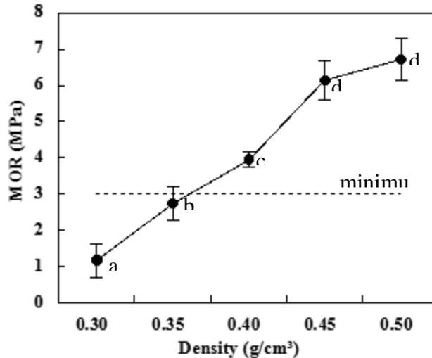
**Fig. 3.** Relationship between density and MOR of low density bagasse particleboard at 15% additive content. Error bars indicate standard deviations. Different letters in the figure indicate that means are significantly different ( $p < 0.05$ )
