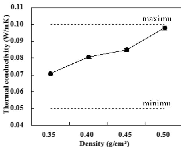
**Fig. 5.** Effects of density on thermal conductivity coefficient of low density bagasse particleboard. Error bars indicate standard deviations
