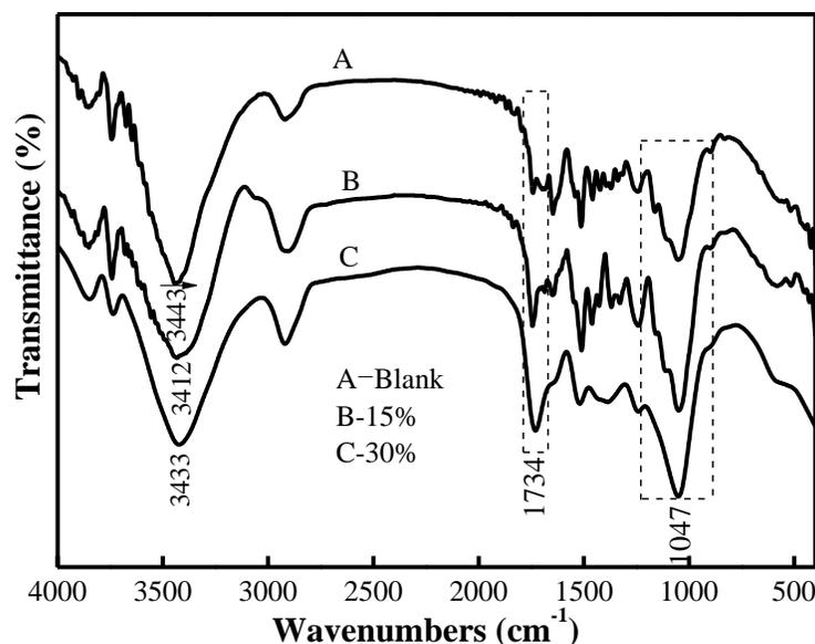
Fig. 6. FTIR spectrum of low density bagasse particleboard with different additive contents
