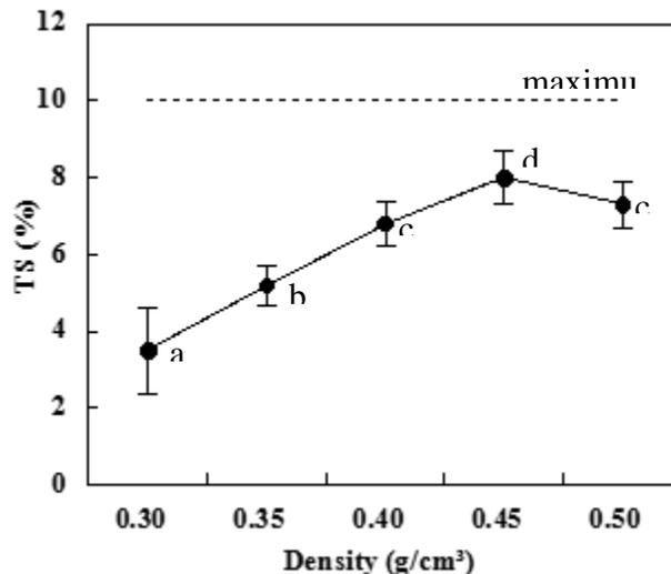
**Fig. 4.** Relationship between density and TS of low density bagasse particleboard at 15% additive content. Error bars indicate standard deviations. Different letters in the figure indicate that means are significantly different ( $p < 0.05$ )
