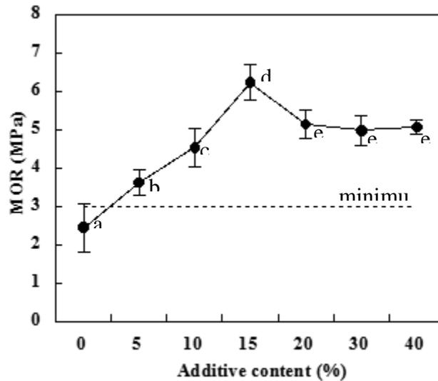
**Fig. 1.** Relationship of low density bagasse particleboard between additive content and MOR at 0.45 g/cm<sup>3</sup> density. Error bars indicate standard deviations. Different letters in the figure indicate that means are significantly different ( $p < 0.05$ )
