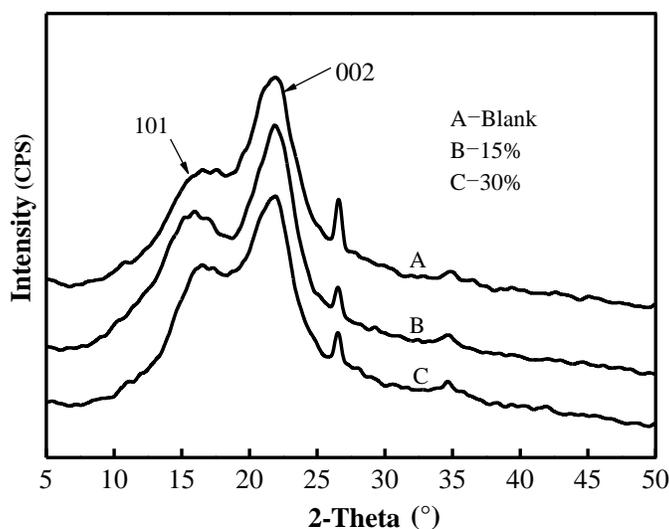
**Fig. 8.** X-ray diffraction spectra of low density bagasse particleboard with different additive content
