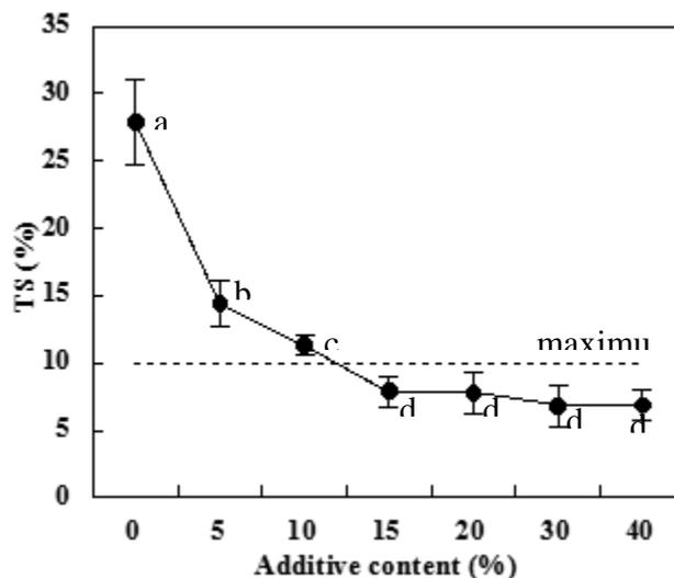
**Fig. 2.** Relationship of low density bagasse particleboard between additive content and TS at 0.45 g/cm<sup>3</sup> density. Error bars indicate standard deviations. Different letters in the figure indicate that means are significantly different ( $p < 0.05$ )
